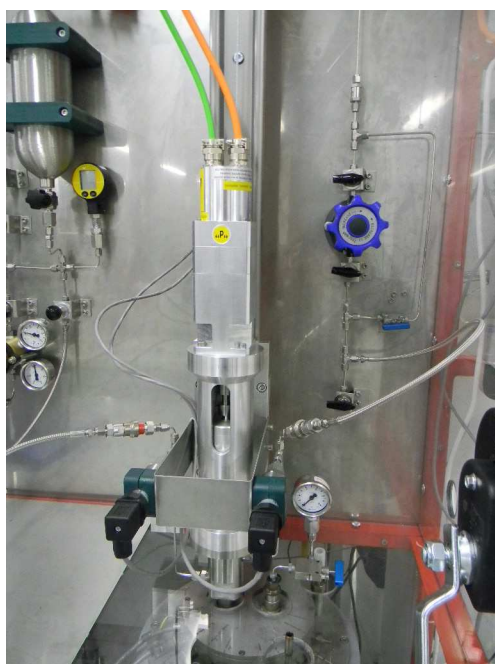
Figure 6 Magnetic stirrer version coupled to the calorimeter
