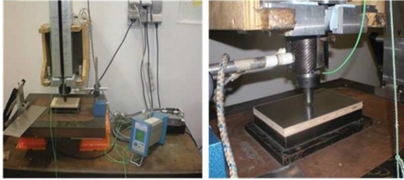
Figure 1. Drop-weight impact test set-up and aluminum wood specimen installed.
