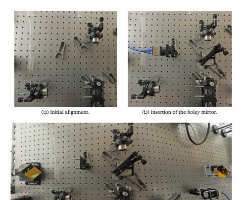
(C) positioning of the fiducials and racetrack alignment.
