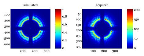
**Figure 3.14:** False colors images of the measurement beam profile after masking and travelling to its detector. Simulated spot and acquired spot are pictured side by side, showing good consistency (intensity in arbitrary units).
