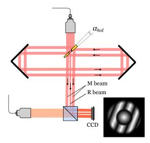
**Figure 3.9:** Simplified layout illustrating the surface parallelism issue:  $\mathcal{M}$  beam tilting is caused by the addition of the racetrack.  $\mathcal{R}$  instead is in single fringe condition.
