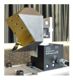
**Figure 3.15:** The wide aperture retroreflector installed onto a tri-axial nanopositioner.
