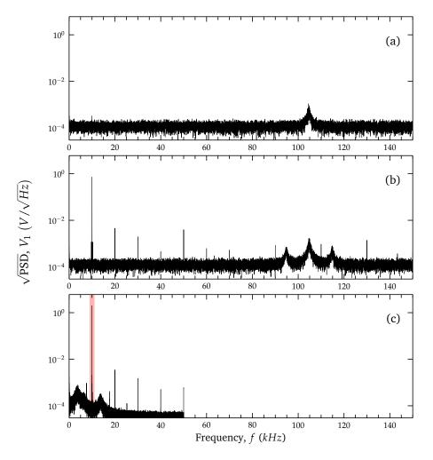
**Figure 3.17**: Spectral analysis of the raw voltage signals coming from the interferometer: (a) spectrum of the signal generated by arm 1 light through  $\mathcal{R}$  path; (b) spectrum of the signal generated by recombination light through  $\mathcal{R}$  path; (c) spectrum of the same signal as acquired by the phasemeter. The useful detection bandwidth is showed in red.
