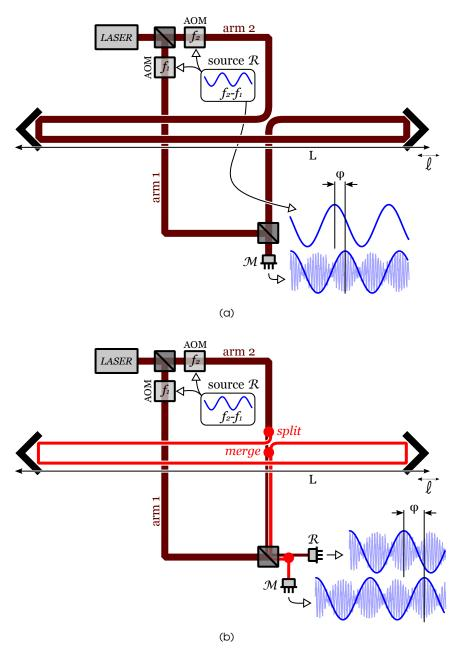
**Figure 2.2:** Simplified layout of a heterodyne displacement interferometer: (a) standard scheme; (b) added cancelable circuit (red path). Folding of arm 2 is required for proper interrogation of the distance *L*.
