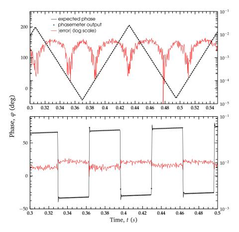
**Figure 3.18**: Response of the phasemeter to reference phase modulations imposed between two wave-generators: (a) 8Hz sawtooth phase modulation with peak-to-peak (pk-pk) amplitude  $A_{pk} = 240^{\circ}$  and (b) 15Hz squarewave with  $A_{pk} = 100^{\circ}$ . The error magnitude (right log scale) is compatible with the numeric limitations produced by single precision floats.
