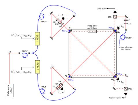
**Figure 1.8**: Optical scheme of the GP2 experimental apparatus. The triple frequency modulation signals can be seen as the inputs to the EOMs. EOM: electro-optic modulator, PBS: polarizing beam-splitter, IBS: intensity beam-splitter, PMOF: polarization-maintaining optical fiber,  $\lambda/2$ , half-wave plate,  $\lambda/4$ : quarter-wave plate, PZT: piezo-electric transducer, F: neutral filter.
