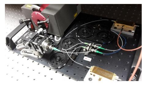
Figure 3.1: Heterodyne source unit mounted on its portable breadboard.
