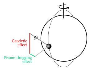
**Figure 1.1:** Simplified representation of a gyroscope orbiting aroud the planet Earth. General relativistic effects on the gyroscope are showed in color: the precessions make its spinning axis change orientation.
