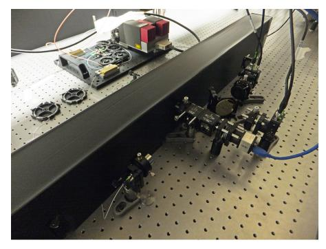
**Figure 4.4:** Picture of the displacement gauge with the racetrack protected by a plastic enclosure.
