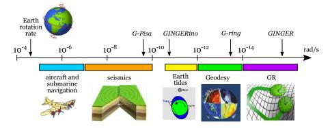
**Figure 1.3:** Orders of magnitude of rotations and ring laser gyroscopes. The sensitivities in measuring rotations achieved by the G-Pisa and the G-ring experiments are indicated, as well as the target sensitivity needed to measure the Lense-Thirring effect.
