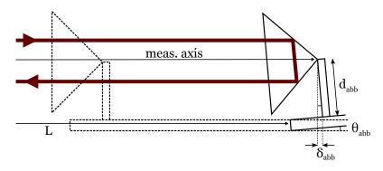
Figure 2.6: Schematic representation of the Abbe error.
