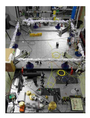
**Figure 1.6:** G-Pisa ring-laser in the horizontal configuration.
