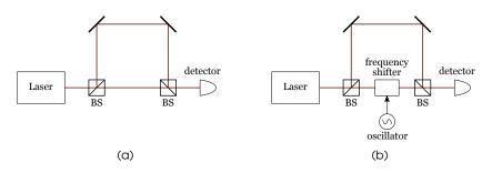
**Figure 2.1:** Comparison between homodyne and heterodyne interferometry: (a) homodyne scheme; (b) heterodyne scheme.
