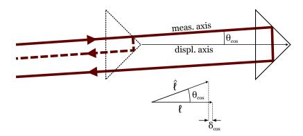
Figure 2.7: Schematic representation of the cosine error.
