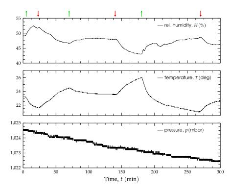
**Figure 4.9:** Monitored ambient parameters over a period of 5h. The arrows at top indicate the instants of activation (up, green) and deactivation (down, red) of the air conditioning system. Data quantization is visible due to the limited resolution of the sensors.
