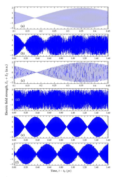
**Figure 3.3:** Simulated optical beating with  $\lambda = 1064 nm$  and  $f_{het}/\nu = 0.01$ . The output at  $\mathcal{R}$  or  $\mathcal{M}$  detector are showed for different optical path configurations and source linewidth values:
