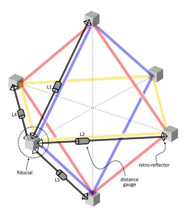
**Figure 1.12:** Simplified schematic of the external metrology truss matched to GINGER in the ochtahedral configuration (for a clearer appearance only one complete vertex is showed).
