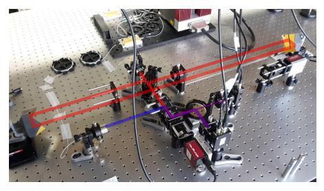
**Figure 3.7:** Displacement gauge under test. The beam paths of arm1 and arm2 are indicated in purple and red respectively.
