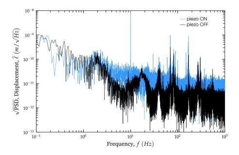
**Figure 4.6**: Noise spectral density of the interferometer with the piezo actuator turned off (bottom curve) and on (top curve). When the actuator is switched on, raising of the mechanical noise floor is clearly visible.
