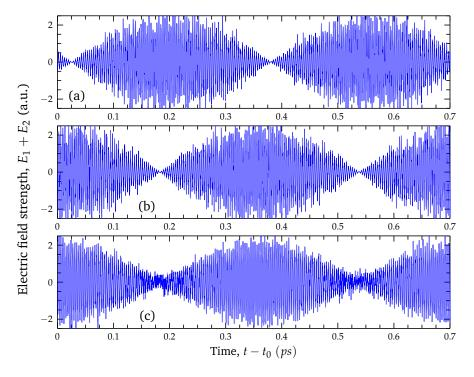
**Figure 3.4:** Simulated optical beating with  $\lambda = 1064 nm$  and  $f_{het}/\nu = 0.01$ . The output at  $\mathcal{R}$  or  $\mathcal{M}$  detector are showed for different optical path configurations in presence of amplitude noise:
