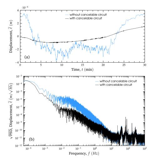
**Figure 4.7:** Comparison between two datasets relative to the same acquisition period. In (a) an extract from the two time series: the smoother one is obtained by applying the lock-in algorithm to  $V_{\rm R}$  and  $V_{\rm M}$ , both optically generated; the other curve results from applying the same algorithm to  $V_{\rm R}$  and  $V_{\rm E}$ , an electrical reference obtained from the RF driver. In (b) the corresponding PSDs are reported.
