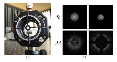
**Figure 3.11:** Pictures of (a) the custom ring mask mounted on a x-y kinematic manual stage and (b) the beam cross-sections before and after masks insertion, showing a good reduction of the unwanted diffraction patterns.
