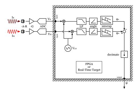
**Figure 2.3**: Schematic representation of the system for interferometric signals acquisition and phase retrieval (lock-in detection).
