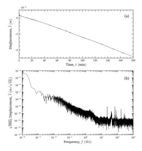
**Figure 4.5**: Monitored displacement in best working conditions over a 3h period: (a) time series and (b) power spectral density.
