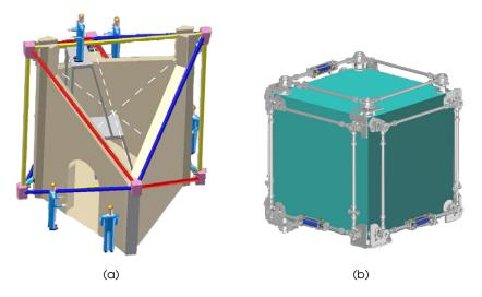
**Figure 1.11:** Representations of the GINGER apparatus: (a) concept drawing of GIN-GER's experimental site after implementation of the octahedral configuration and (b) GINGER in cubic configuration.
