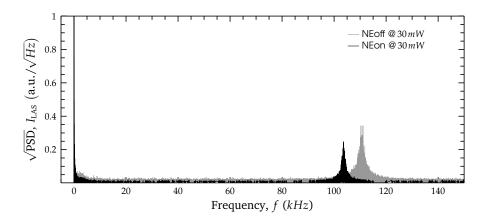
**Figure 3.5**: Source light spectrum near DC: the laser source presents a spurious amplitude modulation at a frequency of about 100 kHz. The peak location and magnitude depend on the output power and on the operation of the noise eater embedded into the laser unit.
