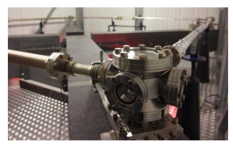
Figure 1.9: Detail of a corner mirror of the GINGERino experiment at LNGS
