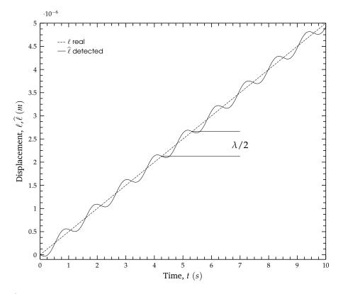
**Figure 2.4**: Output of a displacement gauge affected by cyclic non-linearity: the dashed line represent the ideal interferometer output; the solid curve is the measured displacement (exaggerated).
