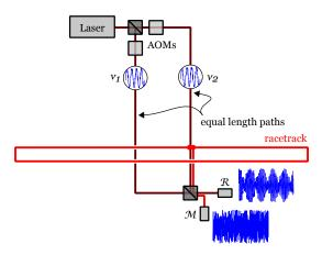
**Figure 3.2:** Reference interferometric configuration for the simulated optical beats. The displayed output refer to a source coherence length of 14m which falls between the actual 4m arms length and the sum of an arm length with the imposed racetrack length 2L = 20m; clearly the loss of coherence due to racetrack travelling nulls beats visibility on the  $\mathcal{M}$  detector.
