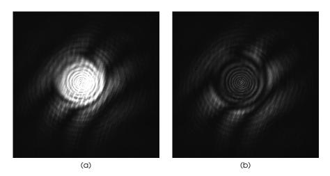
**Figure 3.10:** Picture of the beams cross-sections after recombination: (a) central fringe bright condition and (b) central fringe dark condition. The wedge interference pattern can be clearly distinguished across the outer ring zone (images side is 10 mm).
