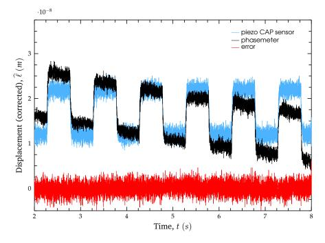
**Figure 4.2**: Gauge output during a positioning test: the fiducial was moved following a squarewave pattern of period 1*s* and pk-pk amplitude 10*nm*.
