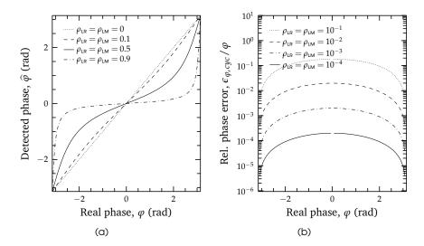
**Figure 2.5**: Simulated cyclic error over a displacement period, computed for different levels of leakage between  $\mathcal{R}$  and  $\mathcal{M}$ : (a) detected phase and (b) relative phase error.
