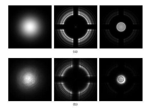
**Figure 3.13:** Comparison between (a) simulated beam cross-sections and (b) acquired beam cross-sections at different locations inside the interferometer. From left to right: collimated beam at exit from the fiber collimators,  $\mathcal{M}$  beam on detector ( $\mathcal{R}$  blocked),  $\mathcal{R}$  beam on detector ( $\mathcal{M}$  blocked).
