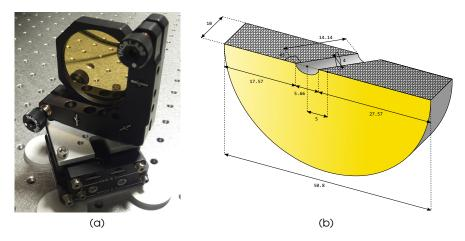
**Figure 3.8**: Wavefront division mirror with central tilted hole and front-back coating: (a) picture of the holey mirror mounted on a 6 dof kinematic manual stage and (b) custom design provided to the manifacturer (all critical dimensions are reported).
