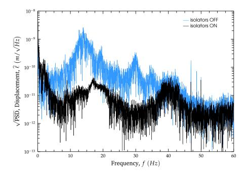
**Figure 4.8**: Responses of the interferometer at rest, with the pneumatic isolators turned off (upper curve) and on (lower curve).
