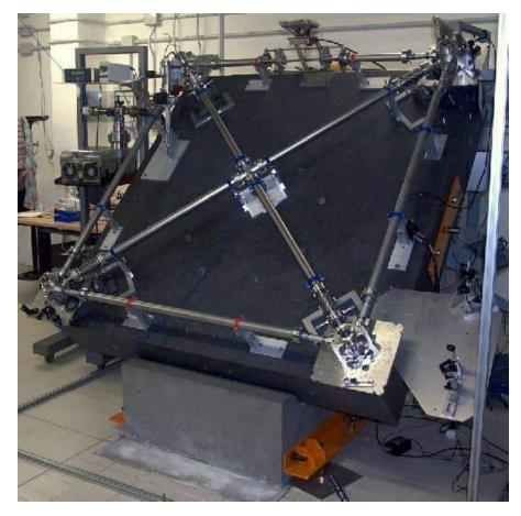
Figure 1.7: GP2 ring-laser installed at INFN-Pisa laboratory.
