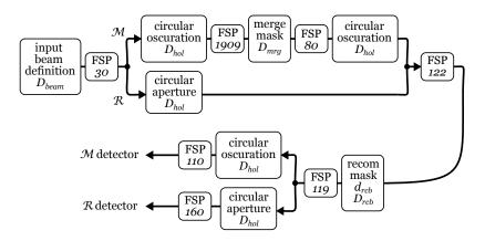
**Figure 3.12**: Displacement gauge POP model: free space propagation (FSP) distances are in *mm*.
