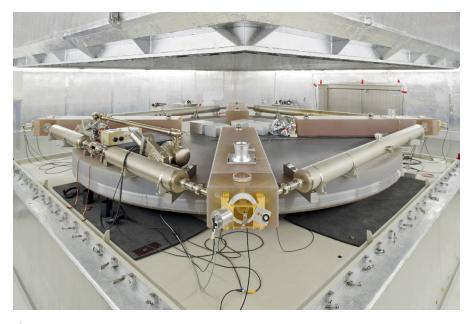
**Figure 1.5**: Picture of the G-ring, showing its semi-monolithic Zerodur structure. The pressure stabilizing vessel can be seen lifted up in the upper part of the picture. Courtesy of U. K. Schreiber.
