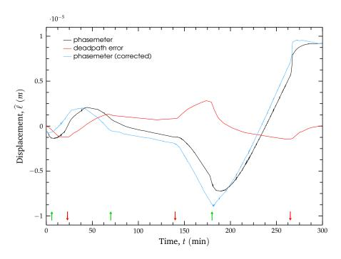
**Figure 4.10:** Monitored displacement over a period of 5h (black), with related deadpath error (red) and resulting corrected trace (blue).
