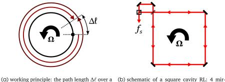
a) working principle: the path length  $\Delta \ell$  over a (b) so single cavity loop is showed.
