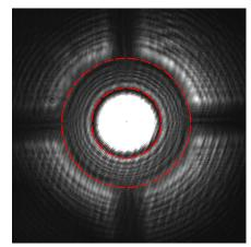
**Figure 3.16:** Beam cross-section of the light coming out from the final recombination BS. Non-beating light fills the ring shaped zone delimited by the mask image (dashed red lines).
