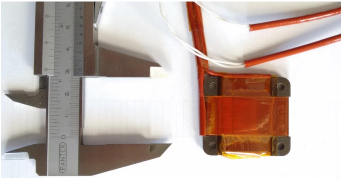
Figure 3-4 Size and appearance of the magnetic probe.
