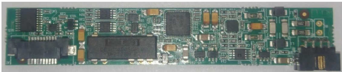
Figure 4-1 ATCA MIMO ISOL module, isolated differential analog fronted board.
