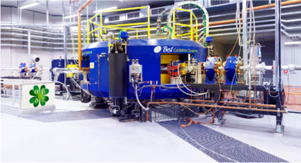
Figure 7.1.: P70 proton cyclotron at the Laboratori Nazionali di Legnaro for the SPES project. The primary proton beam will be accelerated up to the energy of 70 MeV and impinge onto a uranium carbide target, producing several exotic species via proton-induced fission; then, the radioactive nuclei will be reaccelerated by the ALPI super-conductive radio-frequency linear accelerator up to an energy of about 10 MeV/A, to be delivered to the experimental apparatus. Taken from Reference [183].
