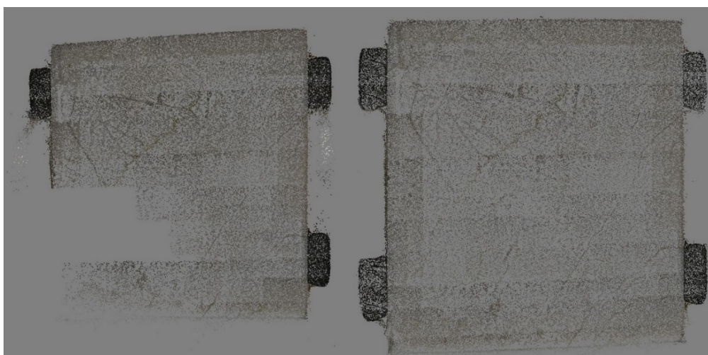
Figure 5. Sample of Orsera stone with lapped surface. Elaboration of the point cloud. On the left the result of the initial alignment, which was very difficult also because this stone has a uniform surface. On the right the successful alignment of the point cloud after the merging of two separate chunks of aligned images.
