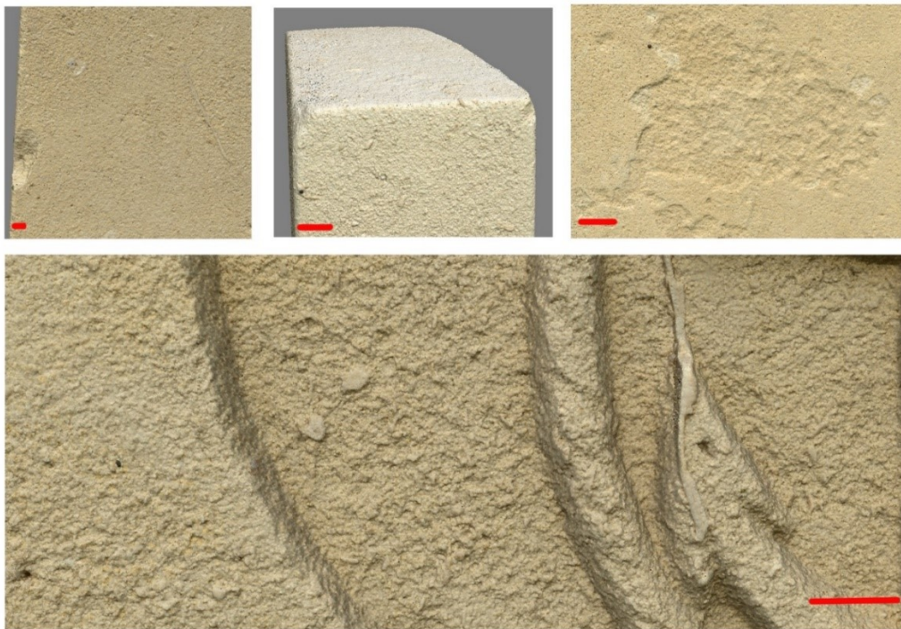
Figure 13. Details of the 3D model of the grave n° 1937 of the Mikra Military cemetery located in Kalamaria (Thessaloniki metropolitan area). This headstone is made of Portland stone and it is aged about 70 years. The red line stands for the unit of 1 cm.
