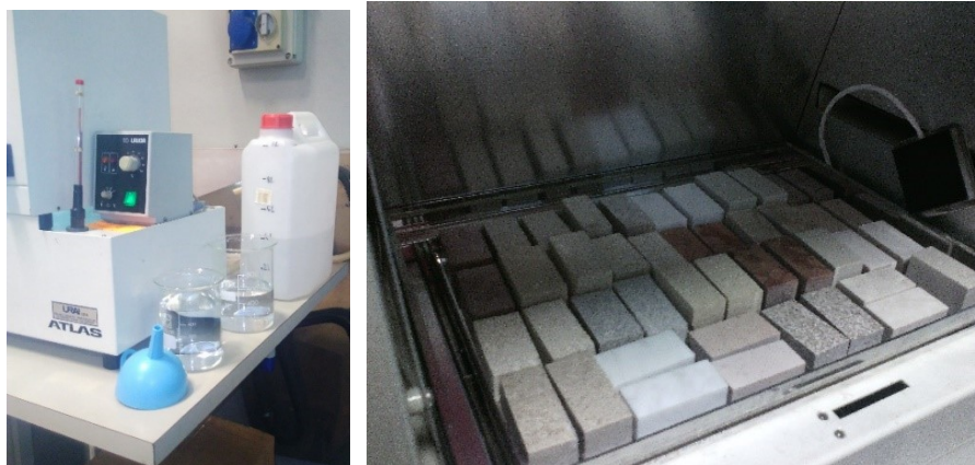
Figure 7. Filling of the climatic chamber (Department of Geosciences) and samples inside.
