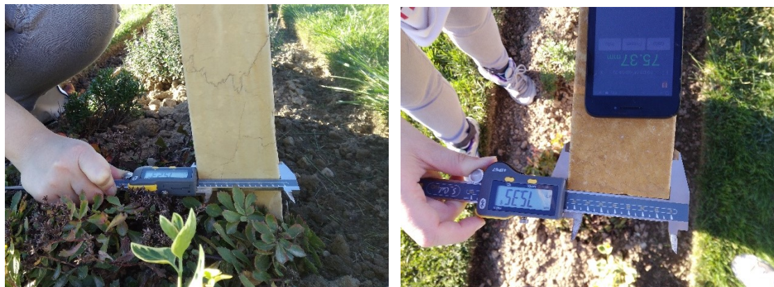
Figure 2. Placement of calipers for recession measurements. In the left a base measurement, always trying to avoid the chipping caused by gardeners), on the right a top measurement, where it is also visible the smartphone recording the measurements through the Sylvac App, which collects the values via Bluetooth®.
