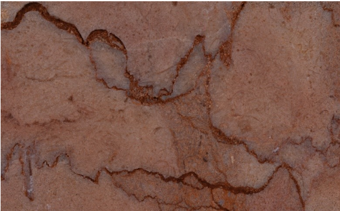
Figure 14. Detail of the 3D model of the Red Verona stone with lapped surface, after 240 aging cycles
