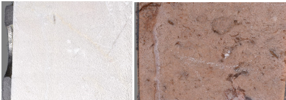
Figure 6. Details of the 3D models of two lapped samples at the end of the accelerated aging test: a sample of Orsera stone is on the left, while a sample of Brown Verona stone is on the right.
