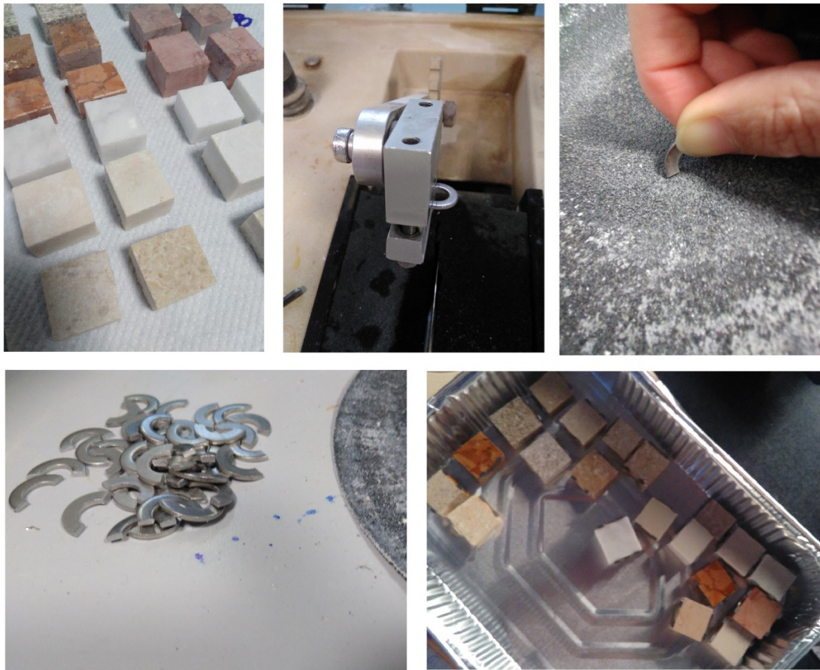
Figure 6. Preparation of the samples in order to be subjected to the accelerated aging tests. View of the samples after the final lapping or polishing stage (a); preparation of reference surface: cutting washers (b), polishing (c-d), view of a set of a sample after attachment to the metal washers to be used as reference surface and final polishing, ready for the accelerated aging tests.
