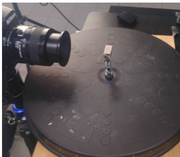
Figure 7. Experimental set up for a quick 3D acquisition of the sample surface. Unfortunately, this method was unsuccessful.
