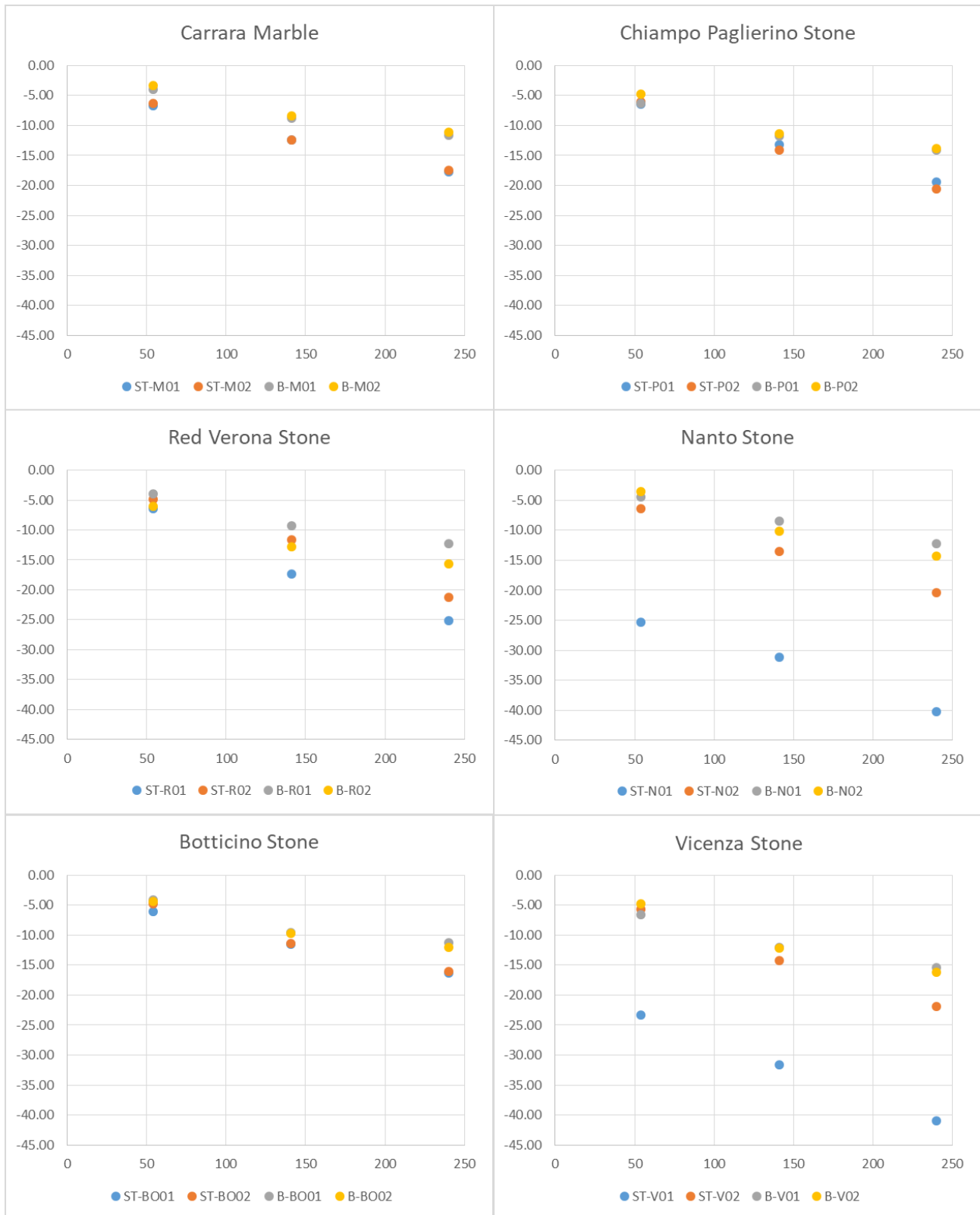
Figure 8. Recession as a function of the number of aging cycles. Samples with label starting with ST (blue and orange symbols) and B (grey and yellow symbols) are those exposed to the rainwater of Stresa and Bologna, respectively. Labels ending with 01 and 02 refer to highly glossy polished samples and lapped samples, respectively.
