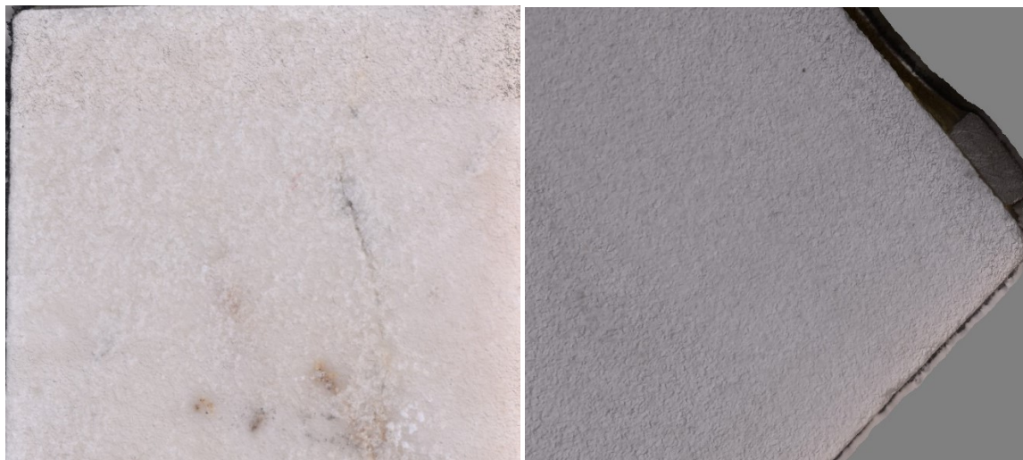
Figure 10. Detail of the 3D models of Botticino stone (on the left, it is possible to see the dolomite crystals) and Carrara marble (on the right)
