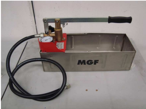
Figure 4.17 - Pump with tank reservoir for pressure tests.
