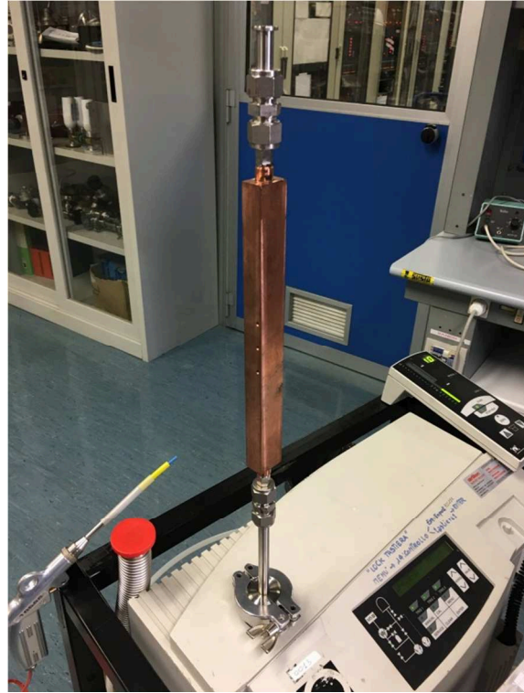
Figure 4.18 - Vacuum Helium leak test operations.
