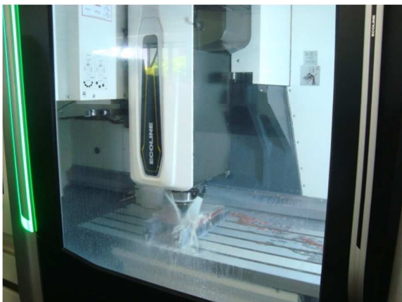
Figure 3.28 - Manifold milling operation
