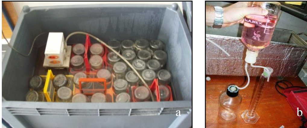
Figure 4.2.3: Lab tests experimental equipment. Mesophilic water bath containing the BMP bottles (a) and manual measurement of the biogas produces through water displacement (b).
