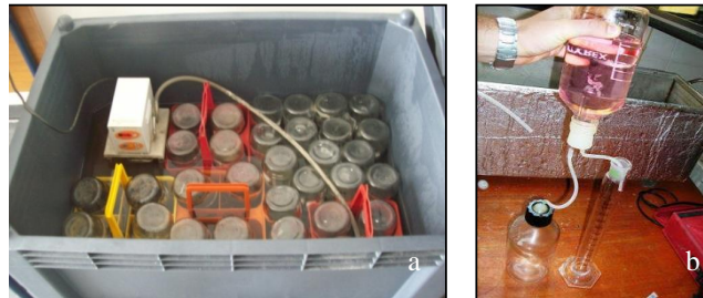
Figure 1.3: Lab tests experimental equipment. Mesophilic water bath containing the BHP/BMP bottles (a) and manual measurement of the biogas produces through water displacement (b).
