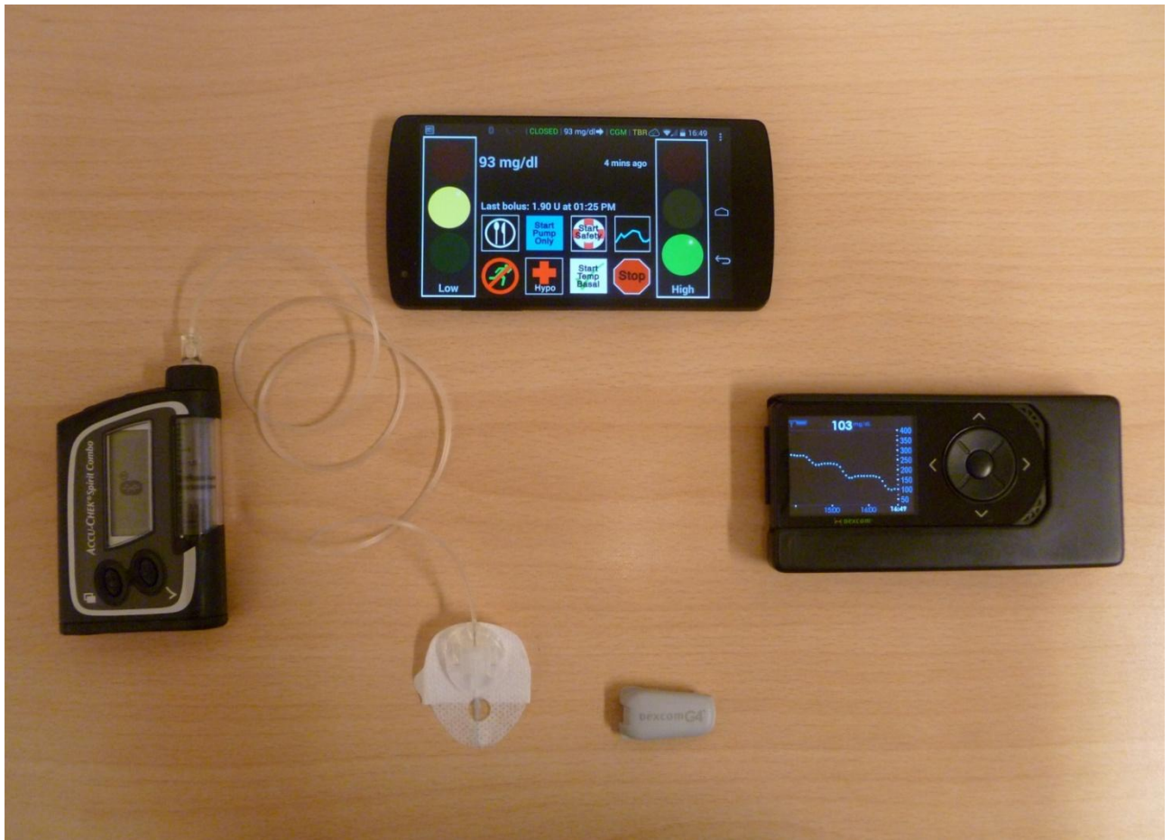
Fig 4: Our artificial pancreas model including DiAs, insulin pump (Accucheck Spirit Combo®, Roche Diabetes Care) and CGM (Dexcom G4®, Dexcom) inserted in relay box to allow Bluetooth communication between receiver and DiAs
