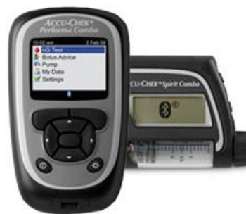
Fig 6: Accucheck Spirit Combo insulin pump. On the left the glucometer and on the right insulin pump. They are equipped with blue tooth connection possibility.
