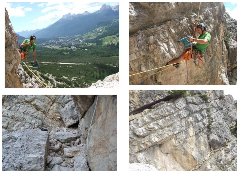
Figure A.3: Setting down of the cable of the pressure transducers to be placed upstream the sharp-crested weir.
