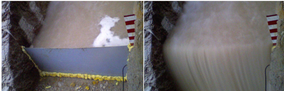
Figure 2.3: Frontal view of sharp-crested weir taken by the time-lapse camera on July 25 th , 2015. The left panel shows the stilling basin partially filled, the right displays the flow discharge over the weir. In both the cases, the water level in the stilling basin is almost steady.
