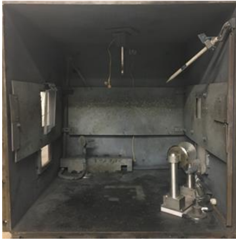
Figure 3: The probe (bottom right corner) mounted in the 1.81 cubic meter explosive blast chamber at the University of Illinois at Urbana-Champaign Explosive Diagnostics Lab.
