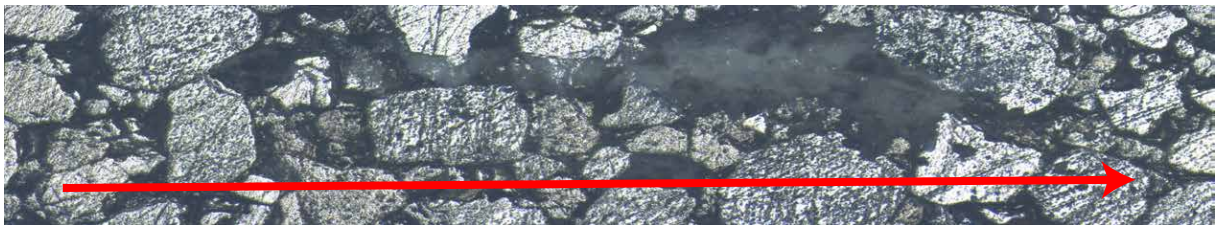
Figure 12.8: Scratch scaling for Mt. Simon sandstone: 6925-U. F_T/\sqrt{2pA} values for scratch length X . The solid line shows the value of fracture toughness, K_c in \text{MPa}\sqrt{m} .
