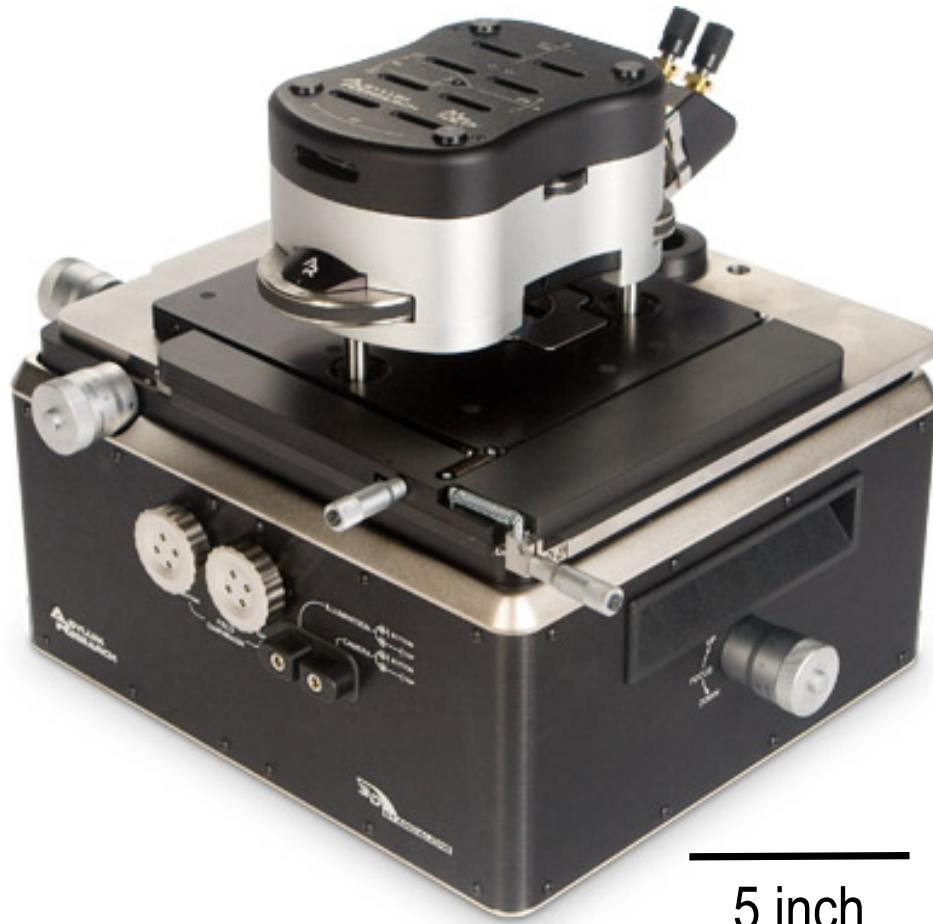
Figure 2.2: Asylum Research MFP-3D TM Stand Alone AFM. Adopted from [44].
