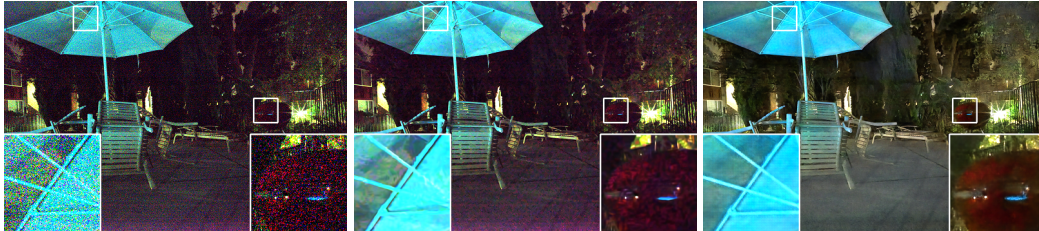
Figure 4.6: An image from the Sony x300 test set. Left: low-light input processed by the traditional image processing pipeline. Middle: same, followed by BM3D denoising. Right: Our result.
