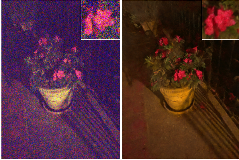
Figure 4.10: Application of a network trained on SID to a low-light raw image taken with an iPhone 6s smartphone. Left: a raw image captured at night with an iPhone 6s with ISO 400, aperture f/2.2 , and exposure time 0.05s. This image was processed by the traditional image processing pipeline and scaled to match the brightness of the reference image. Right: the output of our network, with amplification factor \times 100 .
