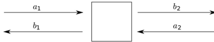
Figure 4.4 2-Port system with input wave ( a_i ) and output wave ( b_i )
