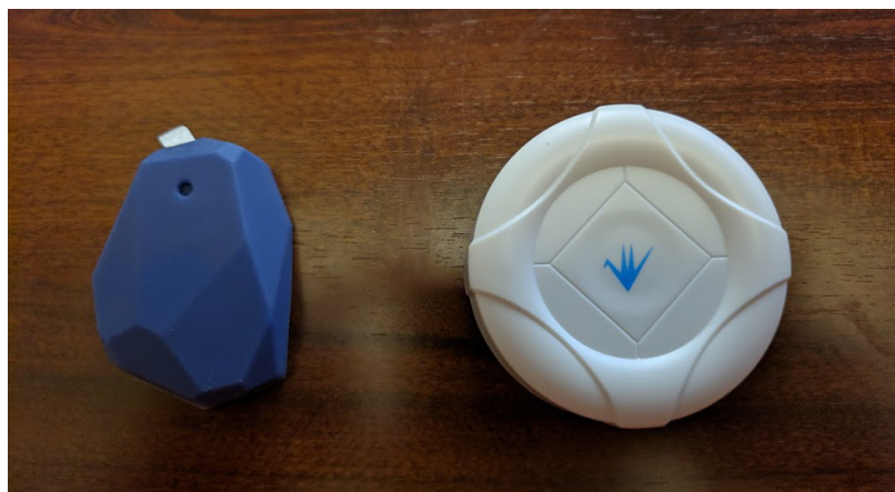
Figure 4.2: A picture of the two different types of beacons used in this work. The beacon on the left is from Estimote and the beacon on the right is from Feasycom beacon.
