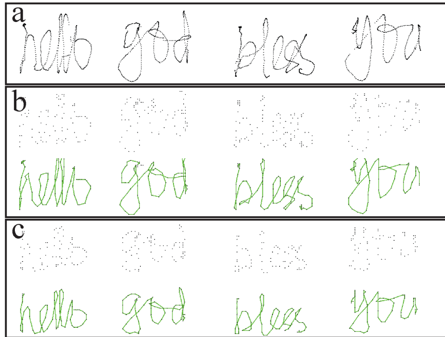
Figure 3.10: We demonstrate the advantages of hand writing with Hybrid HFR Depth. (a)(b)(c) are generated from the same motion sequence. The task is challenging because writing words involves many sharp turns and curves, requiring high frame rate and high accuracy. (b) illustrates using the regular Kinect depth stream (closest point), and (c) illustrates the trace of the Kinect skeleton hand tip. (a) illustrates Hybrid HFR Depth trace, which is of noticeably higher quality due to greater sampling frequency.
