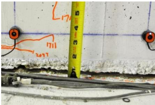
(a) CW2 East flange base separation
