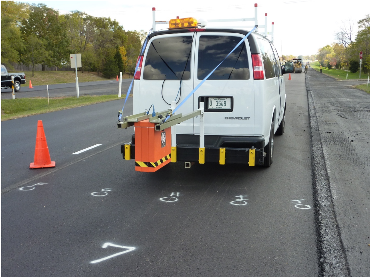
Figure 5-2 GPR data collection.
