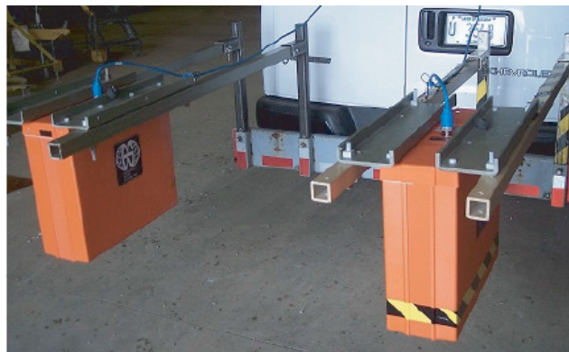
Figure 4-5 Two 2GHz antennas mounted on vehicle (Zhao and Al-Qadi 2017b).
