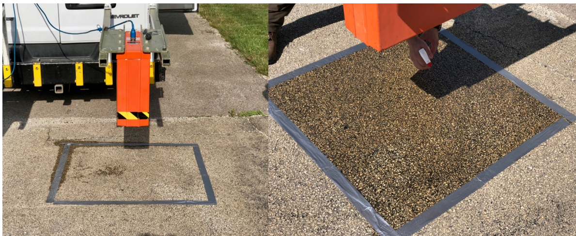
(a) (b) Figure 8-3 Laboratory experiments to analyze the effect of surface moisture on 1 GHz signal: (a) setup of 1 GHz antenna; (b) water sprayed on AC surface
