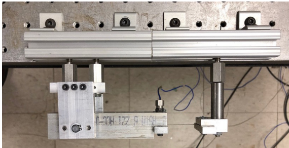
Figure 6.22: (a) The grounded store used in the nonlinear experimental measurements with the fixed-fixed flexure design. (b) Zoomed-in view of the fixed-fixed flexure as attached to the grounded store and grounded pylon.
