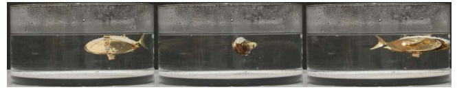
Fig. 10. Frames of the self-folded fish swimming in a water tank under magnetic control
