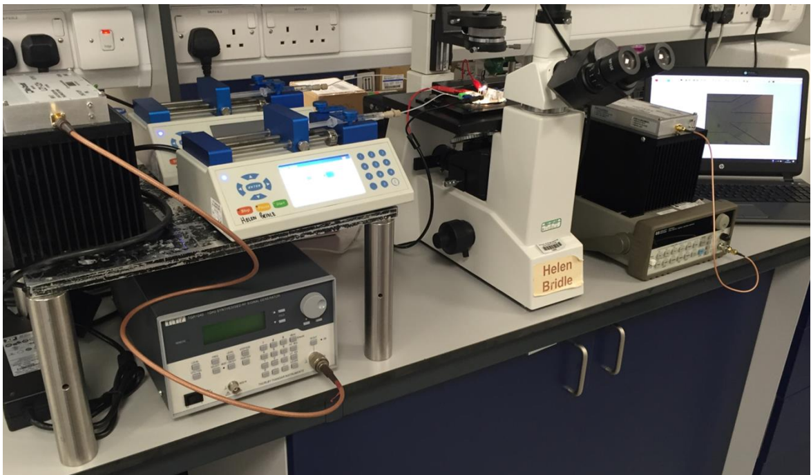
Figure 8.4: Dielectrophoretic chip with all fluidic and electrical connections assembled. Positive pressure from the syringe pumps allowed the introduction of fluid via the sample and buffer inlets, respectively.
