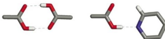
Figure 4.4; identification of possible synthons is the first step. Here is shown a homosynthon (left) and a hetero-synthon (right) [4.18].
