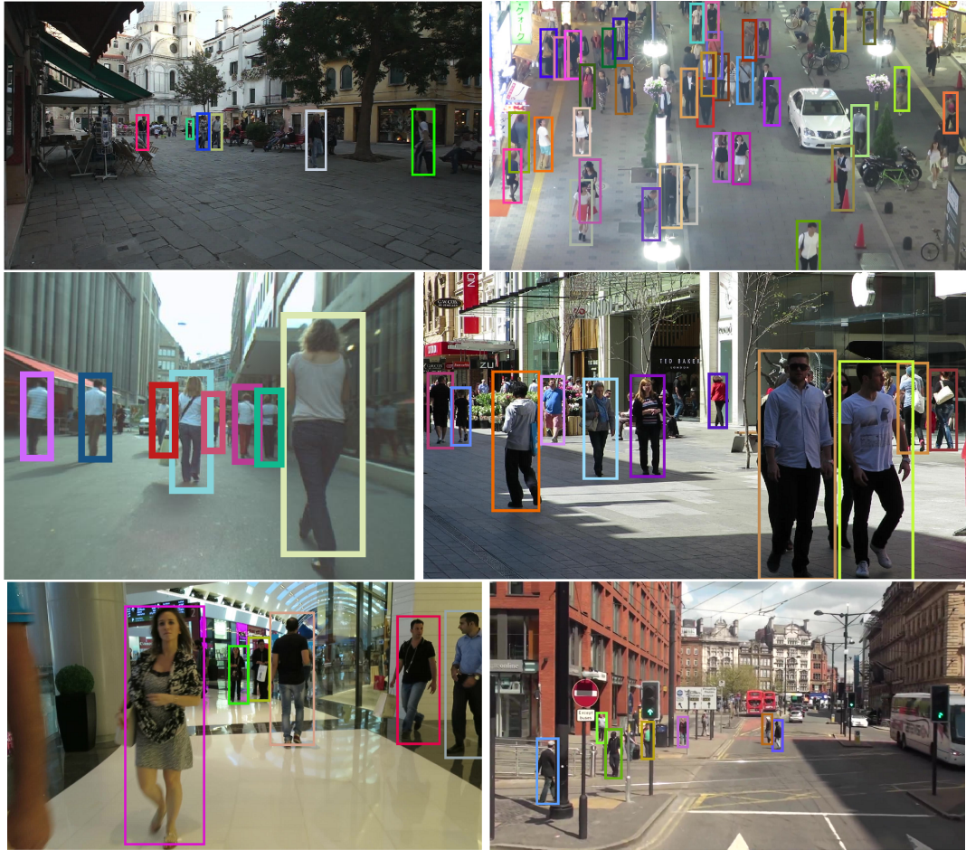
Figure 5.14: Sample results on several sequences of MOT16 datasets, bounding boxes represents the tracking results with their color-coded identities. From left to right: MOT16-01, MOT16-03 (top row), MOT16-06, MOT16-08 (middle row), and MOT16-12, MOT16-14 (bottom row).
