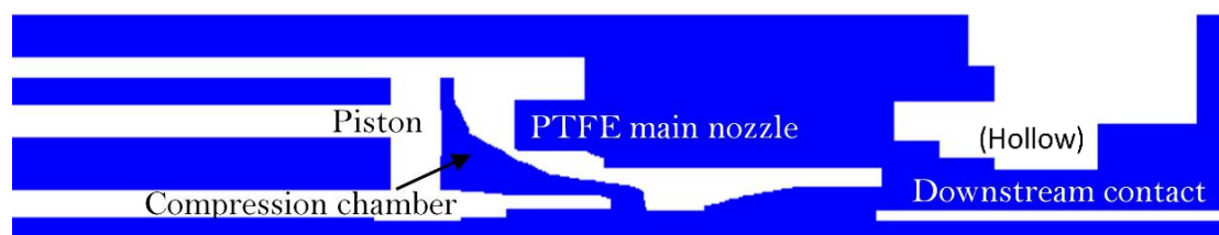
Figure 4.1 Structure of the interrupting chamber of a Puffer 252 kV SF6 circuit breaker.
