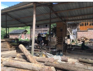
Figure 4: Harvested raw timbers being debarked, processed and sawn into planks and board materials. Guizhou, China [Photograph © Gabriel Tang]
