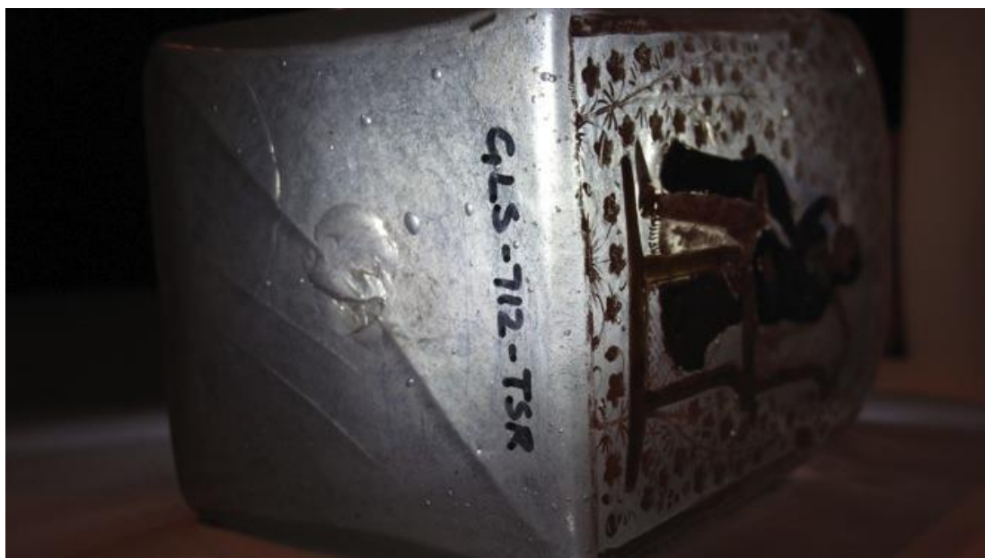
Fig. 120: Detailed view of crizzling on bottle GLS-712-TSR (Tareq Rajab Museum)
