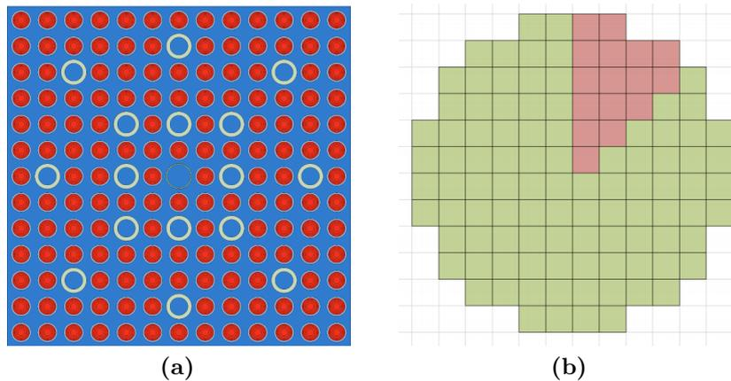
**Fig. 1.** Subassembly sizing: (a)  $13 \times 13$  assembly geometry layout; (b) Schematic of a 112-assembly core, with one octant highlighted.
