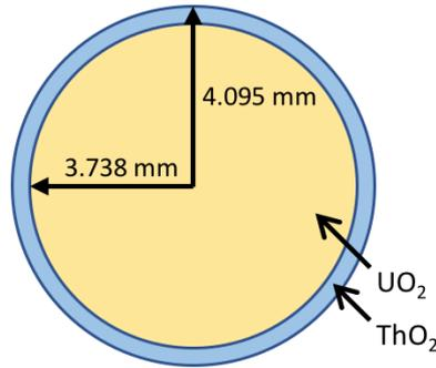
Fig. 2. Configuration of the micro-heterogeneous duplex ThO<sub>2</sub>-UO<sub>2</sub> fuel.
