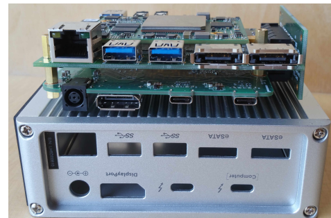
Fig. 1: Thunderbolt dock with FPGA implant, an implementation of our I/O-security research platform
