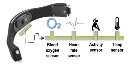
Figure 3.4: Different Sensors in a device called Angel [10]
