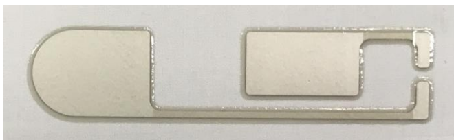
Fig 3. Printing an encapsulation layer onto the interconnections.
