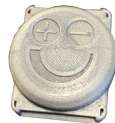
Fig 6. 3D printed circuit cover.
