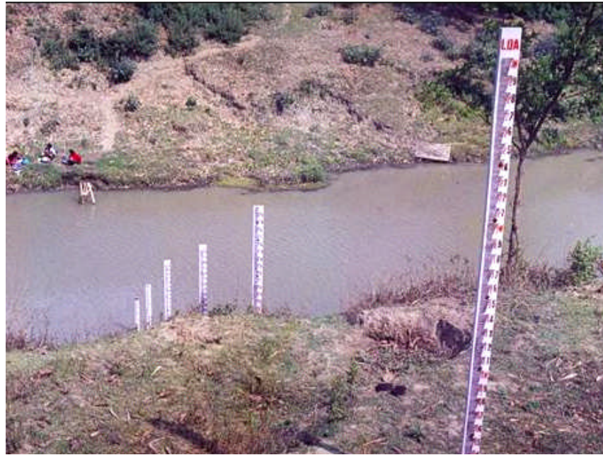
Figure 2.32. Stream gauging station at location on the Iiril River (Source: LDA)
