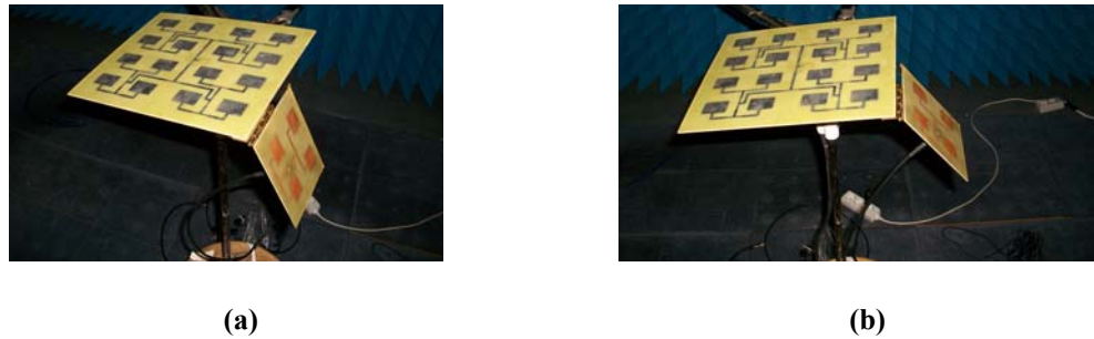
Figure 9: Access and backhaul antenna setup during coupling measurements
