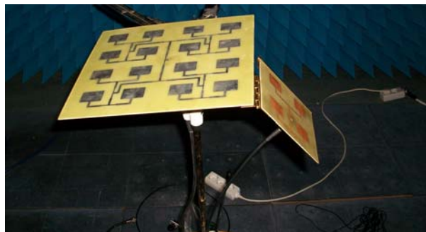
Figure 5.24: Access and backhaul antenna setup during coupling measurements.
