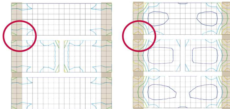
FIG. 4 – Stress shielding scheme: masonry repointed with identical mortar (left) or too rigid mortar (right)
