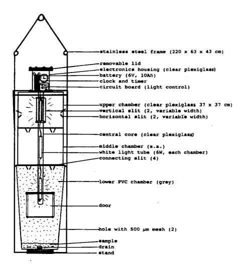
Figure 3. Construction plan of a light trap (Miami-Version).
