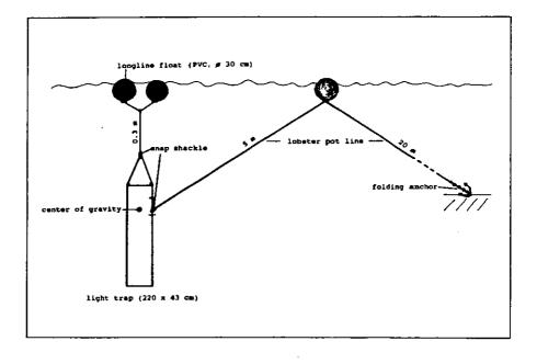
Figure 4. Mooring of a light trap at Conch-Reef during the first sampling period (September 1992).
