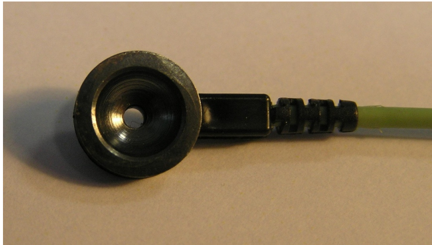
Figure 1.1.4. A standard, clinical, silver/silver-chloride 'cup' electrode. The cup is 9mm in diameter.
