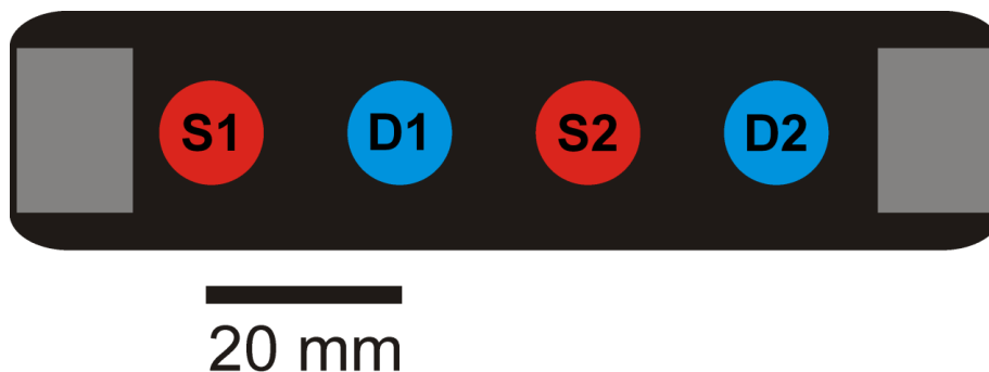
Figure 3.1.7. The simplified, four-channel silicone rubber array design. The red circle represents a source pair (with output at both 690 and 850 nm) and the blue circles represent detectors. The grey regions are velcro pads which allow the array to be strapped to the head. The four channels (and separations) are S1-D1 (20 mm), S1-D2 (60 mm), S2-D1 (20 mm) and S2-D2 (20 mm).
