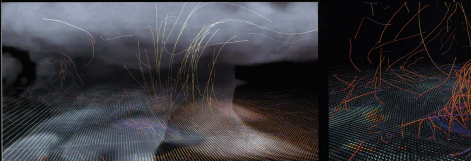
Images from the animated tornado visualization created by NCSA's experimental technologies group. Orange and blue tubes represent the rising and the falling airflow in and around the tornado, which is shown by spheres that are colored according to pressure.
