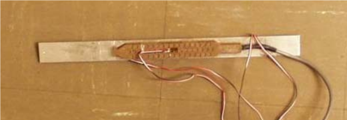
Figure 119. Embedment gage epoxyed to an aluminum bar for cyclic loading
