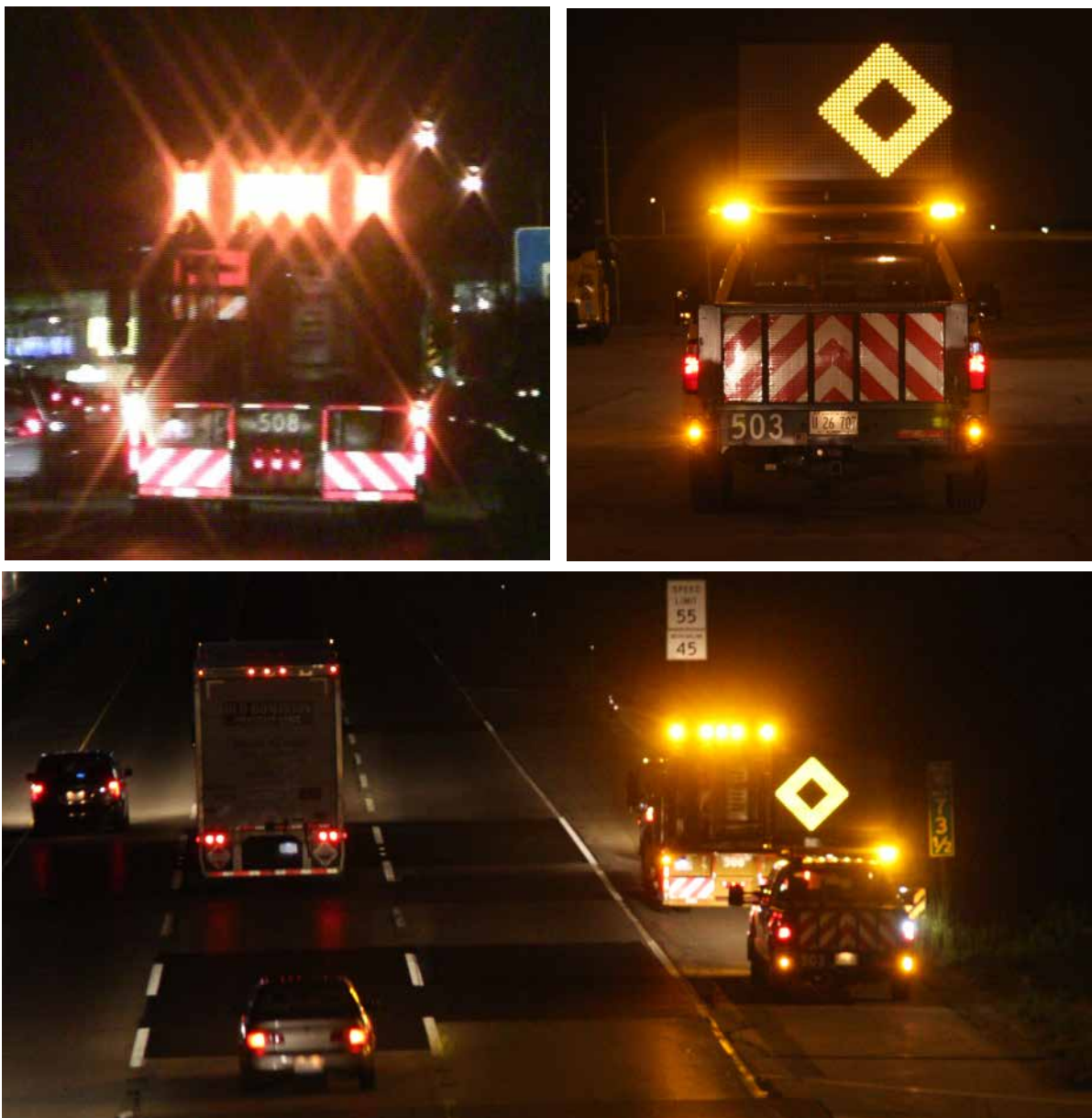
Figure 4.8 Vehicles used to respond to a disabled vehicle on the shoulder: a sign truck with an arrow board in caution mode (top left) and an incident response vehicle displaying a dancing diamond (top right). Both vehicles parked behind a disabled vehicle on the shoulder (bottom).
