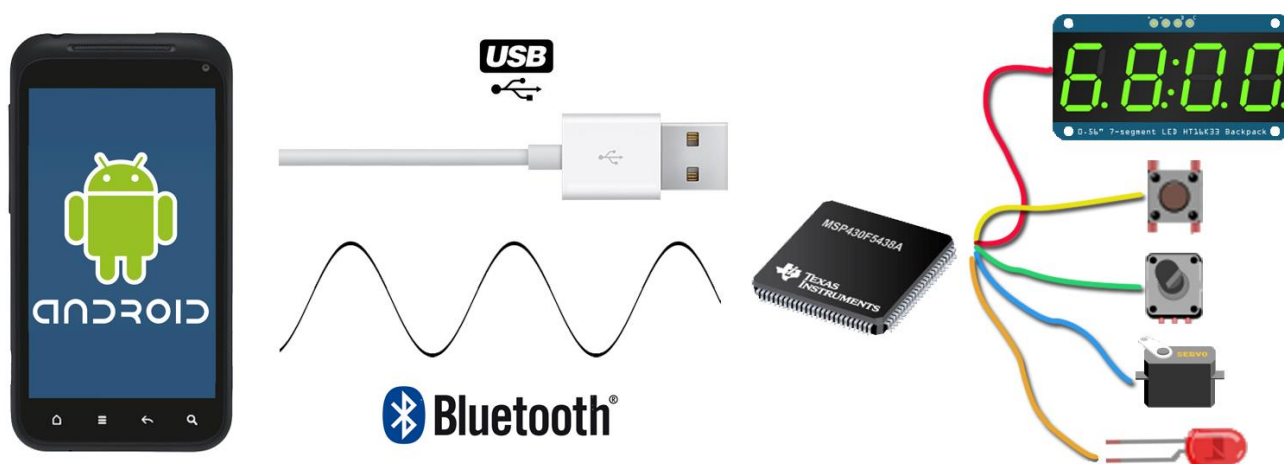
Figure 1: Representation of the different connections between the Android device and the microcontroller
