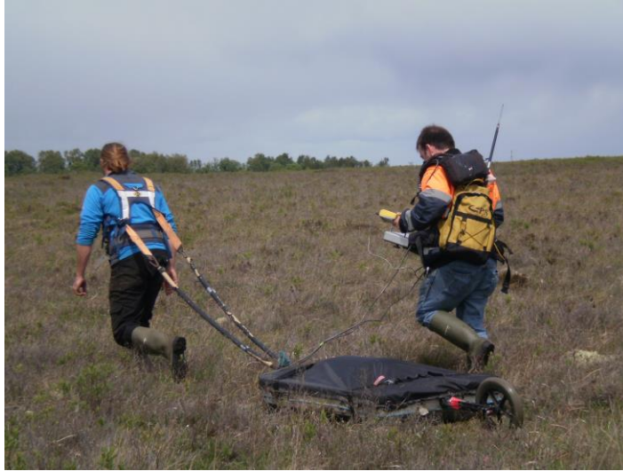
Figure 8. Man-hauling 100 MHz GPR antenna at Roosky
