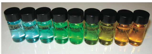
Figure 12. Color changes of \text{Cu}^{2+} solutions ( 0.1 \text{ mol l}^{-1} ) in [\text{ch}]\text{Cl}-\text{H}_2\text{O} mixtures, with water content changing from 100 wt % (blue sample, left) to 27 wt % (yellow sample, right), reproduced with permission from Ref. 66.
