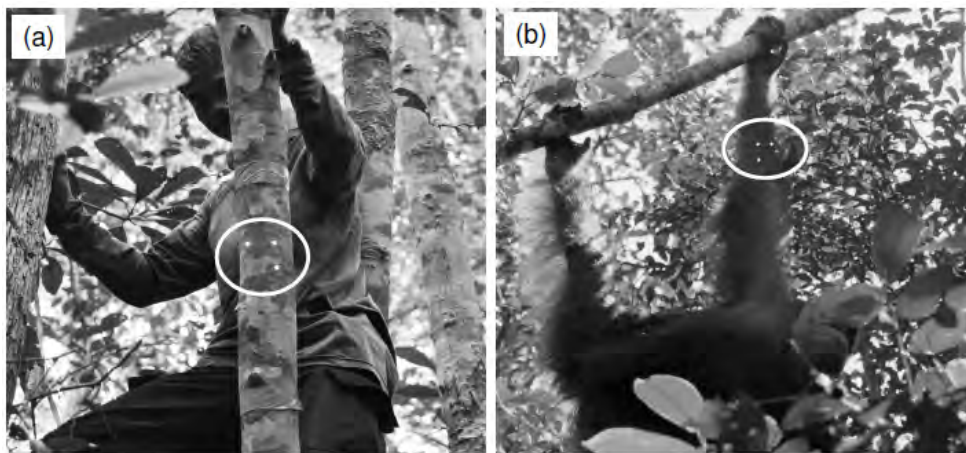
Figure 5.2 – Photographs of a) the validation technique using laser projections on tree branches with known measurements between markers; b) the lasers projected onto the limb of an orangutan.
