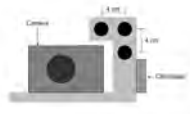
Figure 5.1 – Diagram of the apparatus used to perform the parallel laser technique, which includes an aluminium frame with three lasers set at a known distance (4 cm). A digital camera and clinometer are attached to the frame in a fixed position. The laser beams were regularly calibrated to ensure they were 4 cm apart. The technique was validated using laser projections on tree branches where precise measurements were taken manually.
