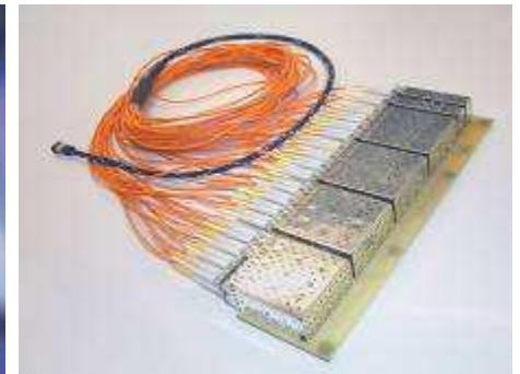
PARA-OPTIX™ Higher Density Ferrules 6 rows of 12 fibres = 72 positions
