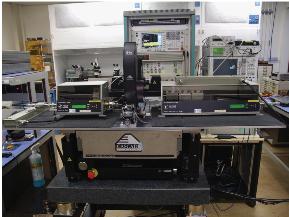
Figure A.1 – Load pull measurement set up installed inside the Payload Division clean room
