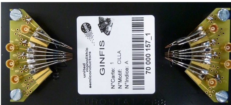
Figure B.3 – Custom made DC probes with SMC male connectors
