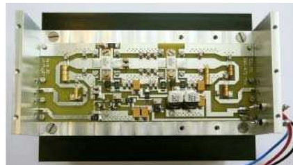
Fig. 3. Purpose-build Power Amplifier module.
