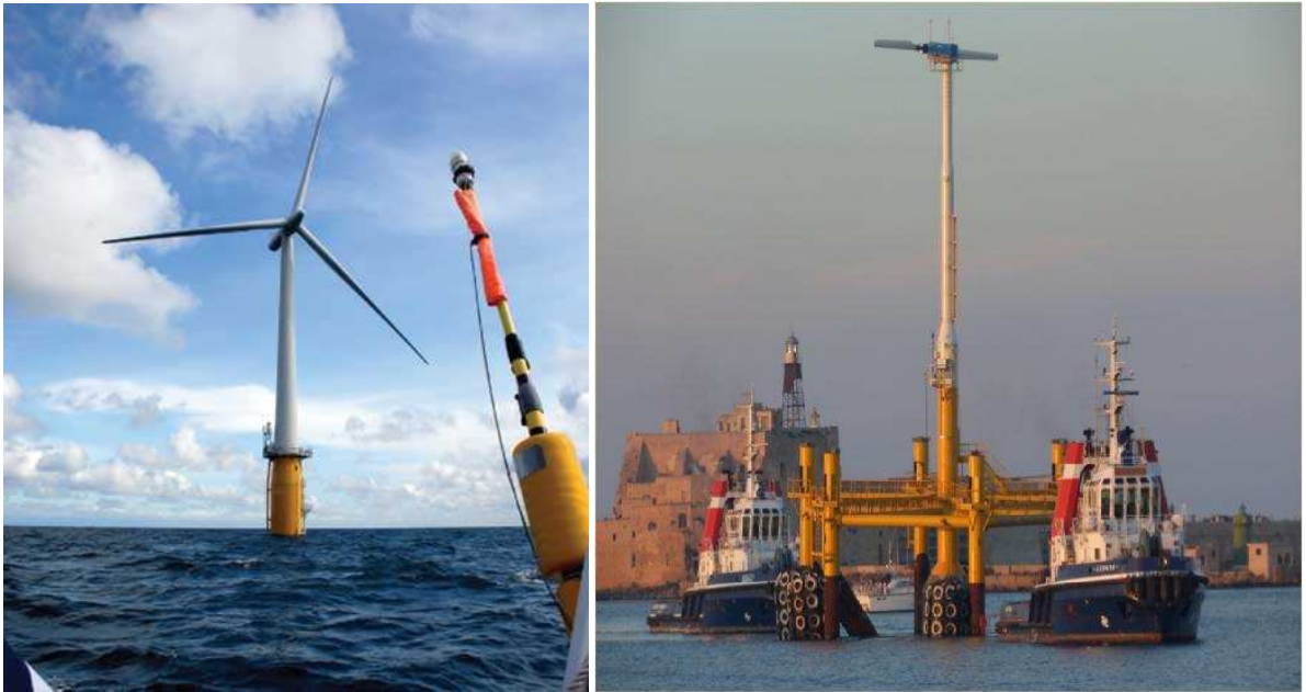
FIGURE 1.4: (a) Hywind prototype, figure courtesy StatoilHydro and (b) Blue H prototype, figure courtesy Blue H
