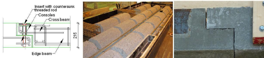
Figure 5.4: Left: detailed drawing of the connection, middle: example on how connection and reinforcement is established in a super-light element, right: example of the detail.
