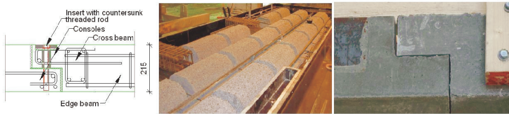
Figure 11: Console connection between super-light indoor pedestrian bridge, on the left production drawing, on the right connection in-situ
