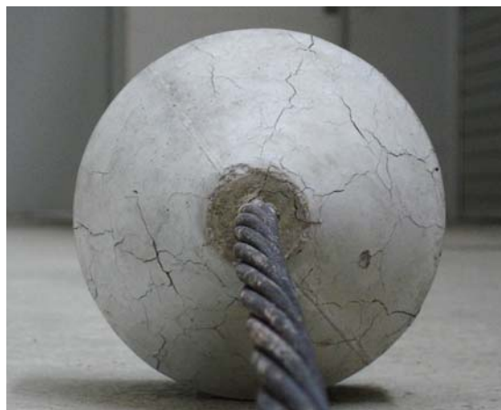
Fig. 9- Conical bond test specimen with prestressing wire and cracks from fire exposure.
