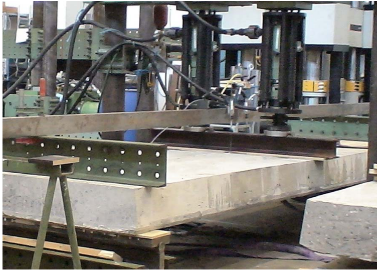
Figure 4.3: Test setup for bending test of super-light element, the steel profile along the element is for deflection measurements.
