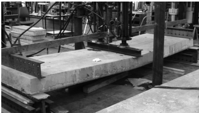
Fig. 5- Bending test rig with a SL-Deck element.
