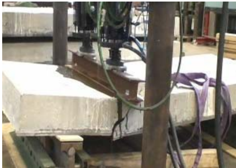
Figure 4.7: Shear test at failure, cracking occurred from tensile stresses with a sudden shear failure.
