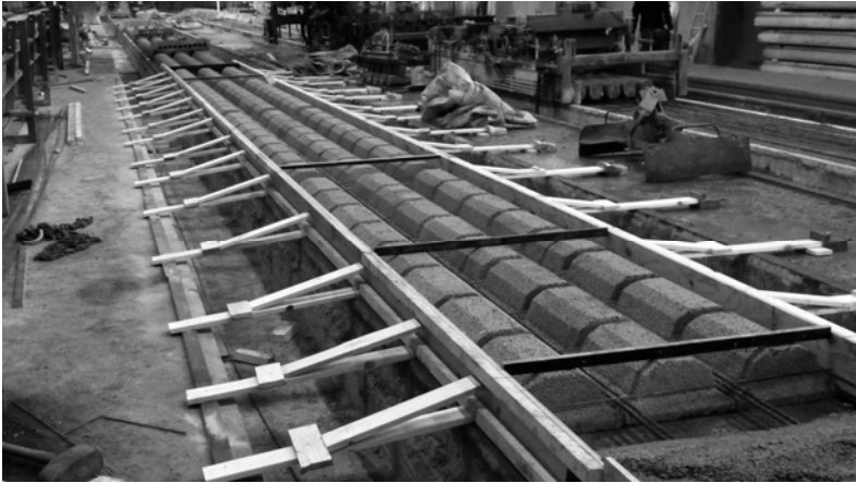
Fig. 1- Principle for a 215 mm (8.5 in) thick, 1.200 m (3.94 ft) wide prototype.
