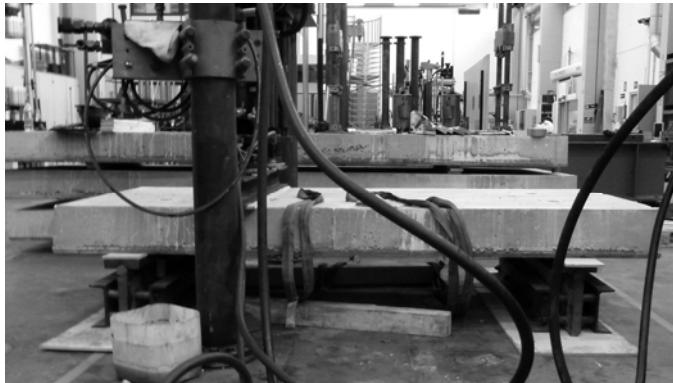
Fig. 8- Shear resistance test with a SL-Deck element.
