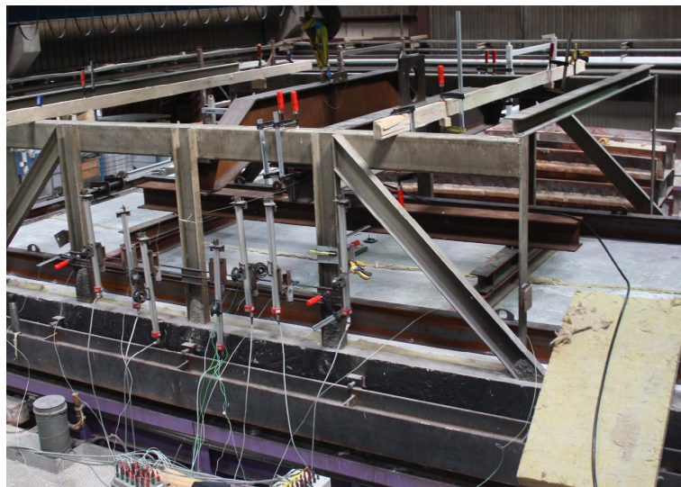
Figure 4.8: Test setup for fire test of super-light element.
