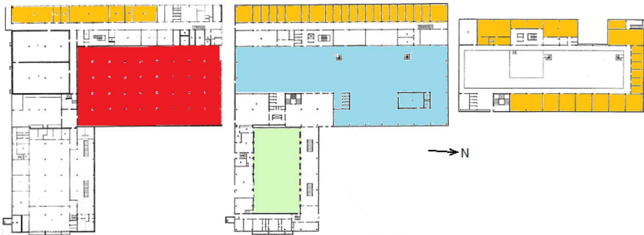
Figure 14: Location of offices at Hvidovre Community Centre, marked in yellow. Floor plan – basement (left), floor plan - ground floor (Middle) and floor plan 1 st floor (right).
