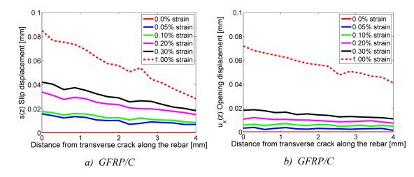
Figure 3-16 Debonding displacement profiles resulting from the transverse crack in GFRP/C showed in Figure 3-10a, a): sliding displacement, slip s(z), and b): opening displacement,  $u_x(z)$ , at different rebar strain levels.
