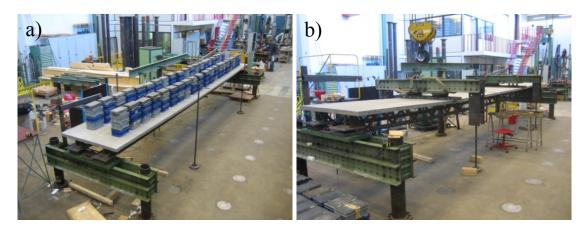
Figure 6-5 Overview of test setups: a) at serviceability limit state (SLS), and b) at ultimate limit state (ULS) loading
