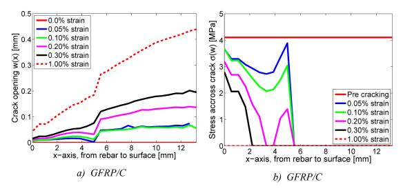
Figure 3-10 a): Crack opening profile for a transverse crack in GFRP/C at different rebar strain levels and b): the corresponding stress transfer across the crack based on the cohesive law for concrete in tension,  $\sigma_c^*(w)$ , shown in Figure 3-2 and fracture mechanical parameters given in Table 3-1.
