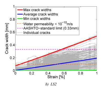
Figure 5-19 Development of crack opening as a function of strain during tensile loading of a): LS1 and b): LS2. The AASHTO crack width limit of 0.33 mm for highway bridges (AASHTO, 2002) is shown for comparison as well as the threshold for water permeability of 10<sup>-10</sup> m/s (Wang et al., 1997).
