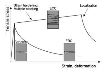
Fig. 4. Schematic tensile stress-strain behavior of cementitious matrices [1].
