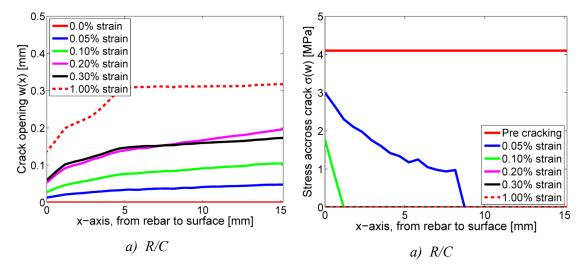
Figure 3-8 a): Crack opening profile for a transverse crack in R/C at different rebar strain levels and b): the corresponding stress transfer across the crack based on the cohesive law for concrete in tension,  $\sigma_{c*}(w)$ , shown in Figure 3-2 and fracture mechanical parameters given in Table 3-1.
