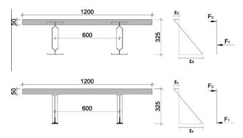
**Fig. 6.** Section view and assumed stress and force distribution of: (a) the Integrally Cast Panel (ICP), b) the modular deck panel (MP). Dimensions are given in mm.
