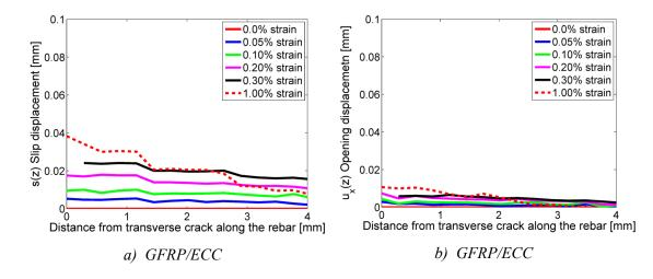
Figure 3-17 Debonding displacement profiles resulting from the transverse crack in GFRP/ECC showed in Figure 3-10b, a): sliding displacement, slip s(z), and b): opening displacement,  $u_x(z)$ , at different rebar strain levels.
