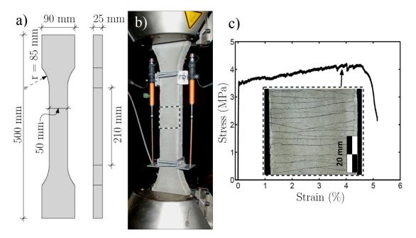
Figure 2-5 a): Geometry of an ECC dog-bone shaped specimen, b): direct tension test setup including supports and LVDT's, and c): example of tensile stress-stain response of an ECC specimens and the resulting crack pattern at approximately 4% strain.
