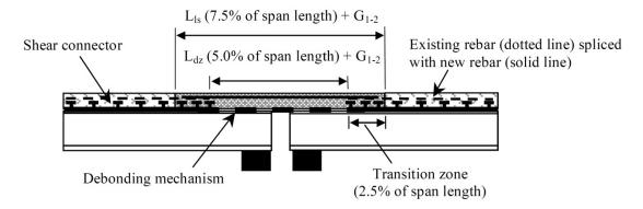
Figure 5-2 Schematic of the ECC link slab implemented in Michigan (Lepech and Li, 2005)
