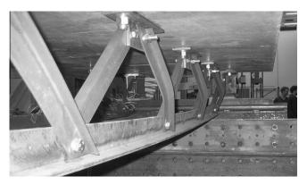
Fig. 19. Buckling of compression diagonals in specimen MP1.
