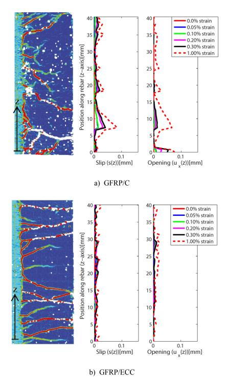
Figure 3-13 Debonding displacement profiles, slip s(z), and opening,  $u_x(z)$ , along the rebar (z-axis) in a): GFRP/C specimen and b): GFRP/ECC specimen at different strain levels.
