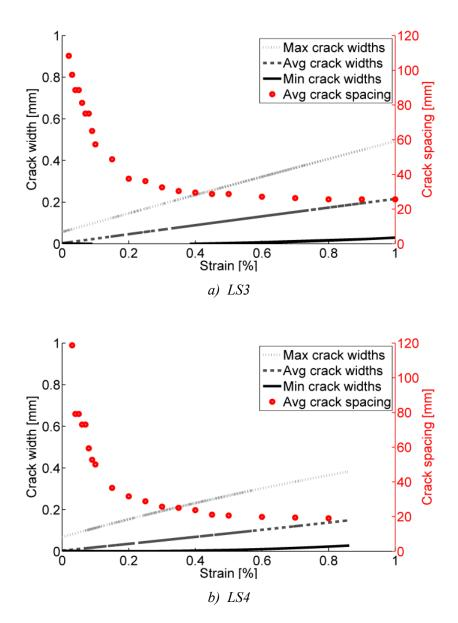
Figure 5-22 Average crack spacing in comparison to maximum, average and minimum crack widths compared with development of crack spacing as a function of tensile strain for a): LS3 and b): LS4.
