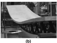
Fig. 20. Deformed shape of specimen MP2 during (a) and after (b) ULS loading.
