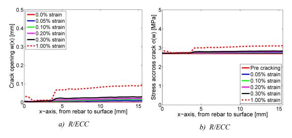
Figure 3-9 a): Crack opening profile for a transverse crack in R/ECC at different rebar strain levels and b): the corresponding stress transfer across the crack based on the cohesive law for ECC in tension,  $\sigma_{ECC}(w)$ , shown in Figure 3-2 and fracture mechanical parameters given in Table 3-1.
