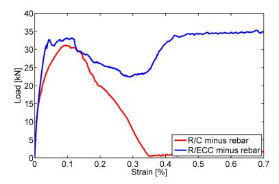
Figure 4-17 The concrete and the ECC contribution in the composite response of R/C and R/ECC respectively.
