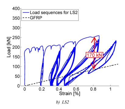
Figure 5-13 Structural response of the active middle part of the link slab a): LS1 and b) LS2. For comparison the response the bare GFRP reinforcement is also shown.
