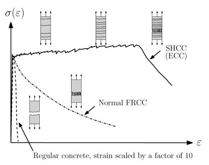
Figure 2-1 Schematic comparison of the stress-strain ( $\sigma$  -  $\varepsilon$ ) response of ductile SHCC, typical strain softening FRCC and brittle concrete under tensile loading.
