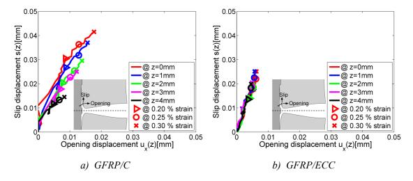
Figure 3-19 Local sliding displacement, slip s(z), Vs. opening displacement,  $u_x(z)$ , of the debonding zone for tensile stain of the reinforcement up to 0.3 % at different distances along reinforcement for a): GFRP/C and b): GFRP/ECC. Markers depict strain levels: 0.20 %, 0.25 % and 0.30 %.
