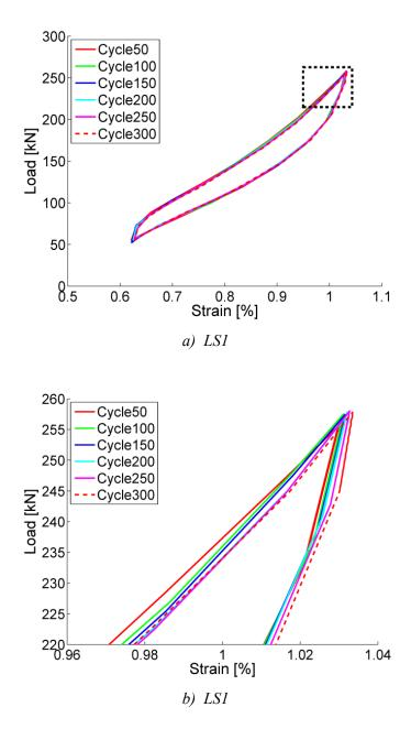
Figure 5-15 Load-strain hysteresis from cyclic testing of LS1. a): overall cyclic response and b): enlarged crest of the hysteresis.
