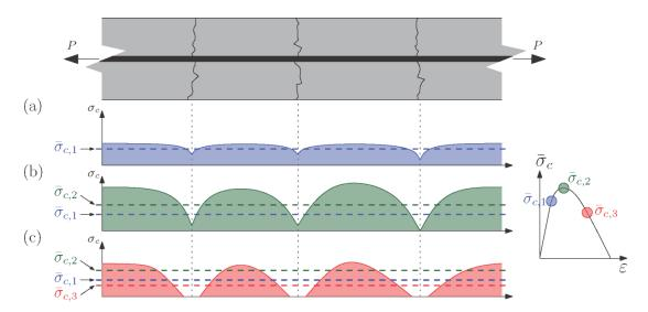
Figure 4-18 Schematic representation of the stress distribution and average stress in concrete in a reinforced concrete element: a) initially after crack formation  $(\overline{\sigma_{c,l}})$ , b) at maximum average stress  $(\overline{\sigma_{c,2}})$  and c) at decreasing average stress  $(\overline{\sigma_{c,3}})$ .
