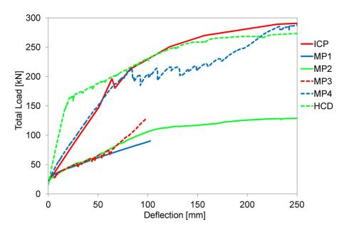
Figure 6-9 Total load applied versus mid-span deflections for specimens MP1, MP2, MP3, MP4, ICP and a hollow core deck panel (HCD).
