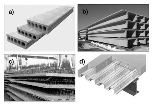
Fig. 1. Commercially available floor systems: (a) hollow core decks [19], (b) double T-deck elements [20], (c) filigree slabs with embedded lattice stirrup ridges [21], and (d) concrete on a pan deck supported by a steel joist [22].
