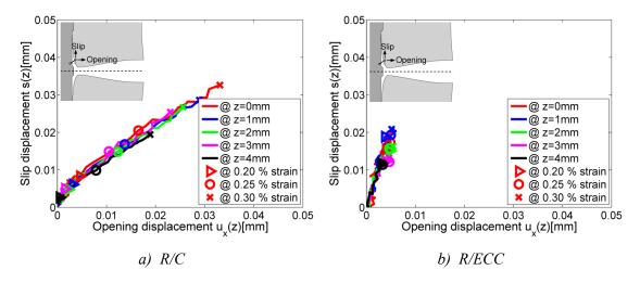
Figure 3-18 Local sliding displacement, slip s(z), Vs. opening displacement,  $u_x(z)$ , of the debonding zone for tensile stain of the reinforcement up to 0.3 % at different distances along reinforcement for a): R/C and b): R/ECC. Markers depict strain levels: 0.20 %, 0.25 % and 0.30 %.
