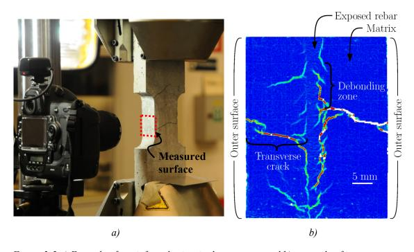
Figure 3-5 a) Example of a reinforced prism in the test setup and b): example of image correlation analysis (DIC), blue color indicates zero deformation while color changes depict principle strain intensities (indicating a crack or slip) on the measured surface (see B-B in Figure 3-4).
