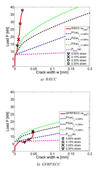
Figure 3-23 Load-crack opening results for a): R/ECC and b): GFRP/ECC in comparison to the three variations of the analytical solutions for the load-crack opening relationships given by equation 3.16 (P1, P2 and P3). Test results are shown up to a rebar strain of 0.3 % with a: triangle, cross, circle and square markers indicating: 0.05%, 0.1%, 0.2% and 0.3% rebar strain respectively.
