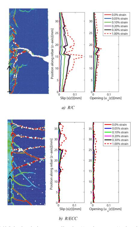
Figure 3-12 Debonding displacement profiles, slip s(z), and opening,  $u_x(z)$ , along the rebar (z-axis) in a): a R/C specimen and b): a R/ECC specimen at different strain levels. Vertical dotted line in a) shows the position along the reinforcement where slip measurements changed direction.
