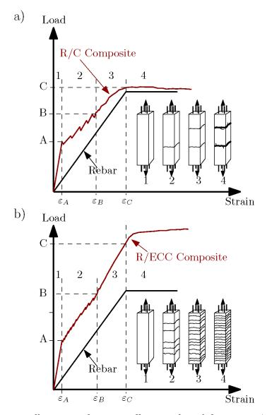
Figure 4-1 Schematic illustration of tension stiffening and crack formation: a) shows R/C and b) shows R/ECC. "A" and  $\varepsilon_A$  are load and corresponding strain of first crack respectively, "B" and  $\varepsilon_B$  are load and strain at crack saturation / stabilized response respectively, "C" and  $\varepsilon_C$  are load and strain at yielding of reinforcement respectively.
