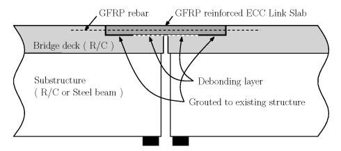
Figure 5-3 Proposed GFRP reinforced ECC link slab concept.
