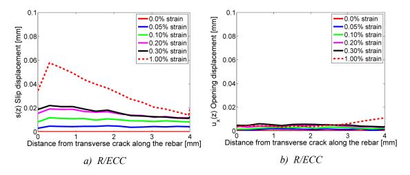
Figure 3-15 Debonding displacement profiles resulting from the transverse crack in R/ECC showed in Figure 3-8b, a): sliding displacement, slip s(z), and b): opening displacement,  $u_x(z)$ , at different rebar strain levels.
