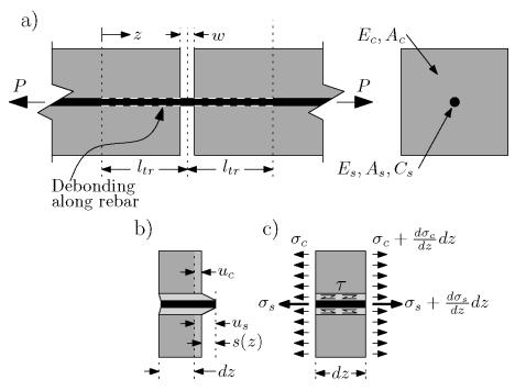
Figure 3-1 a): Schematic illustration of a single transverse crack in a reinforced concrete member, b): displacements in a infinitely small reinforced element (dz) and c): corresponding forces acting on the infinitely small element.
