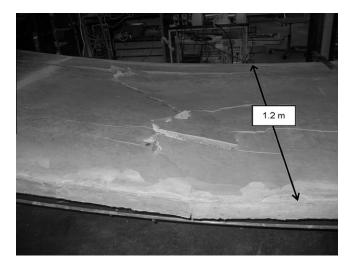
Fig. 18. Compression failure at mid-span of ICP2.
