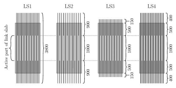
Figure 5-9 Plane view of rebar layout in all link slabs. Dimensions are given in mm.
