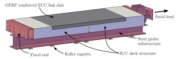
Figure 5-7 Test setup with link slab bridging the two adjacent representative bridge decks.
