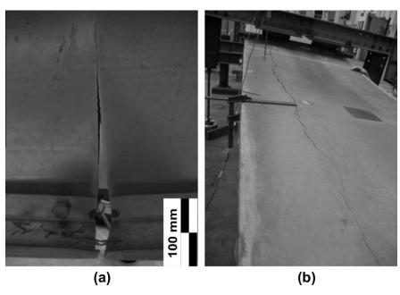
Fig. 17. Failure of specimen ICP1, (a) crack in the steel substructure and (b) a subsequent failure of the ECC deck.
