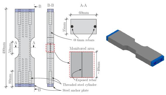
Figure 3-4 Geometry and layout of reinforced prism used to evaluate the rebar-matrix interface in tensile loading.
