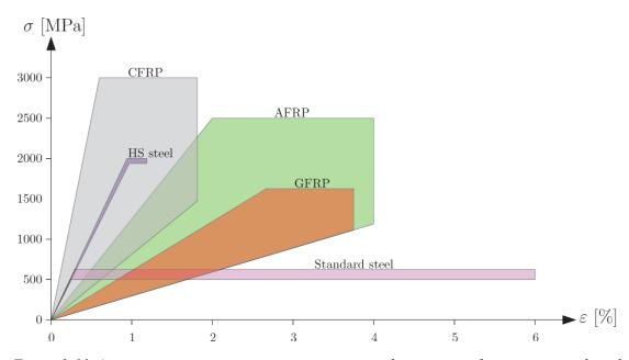
Figure 2-11 Approximate stress-strain response ranges of various reinforcement types based on Model code 2010 (fib, 2010).
