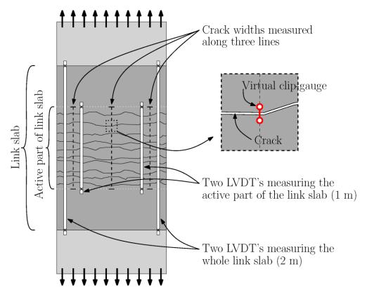
Figure 5-12 Schematic view of measurements taken on top of link slab during testing.
