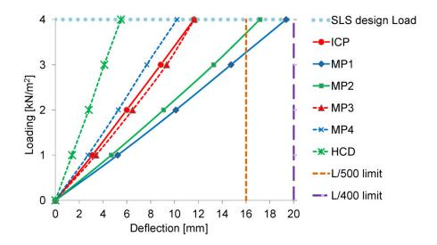
Figure 6-7 Comparison of mid-span deflection of specimen MP1, MP2, MP3, MP4, ICP and HCD as a function of the applied load.
