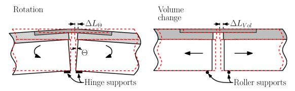
Figure 5-24 Schematic of the expected deformations in the link slab.
