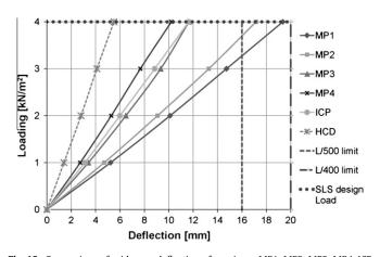
**Fig. 13.** Comparison of mid-span deflection of specimen MP1, MP2, MP3, MP4, ICP and HCD as a function of the applied load.
