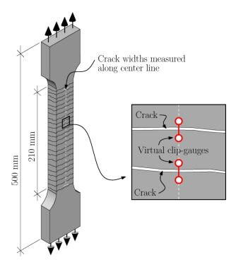
Figure 2-6 Schematic of a dog-bone shaped specimen used to characterize ECC's tensile behavior. Utilizing a Digital Image Correlation (DIC) system, the close-up view shows positioning of virtual clip gages used to monitor the crack opening displacements.
