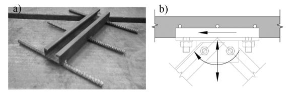
Figure 6-4 a) Cast-in anchor. b) Resultant forces expected in cast-in anchor, forces shown in vertical and longitudinal direction.
