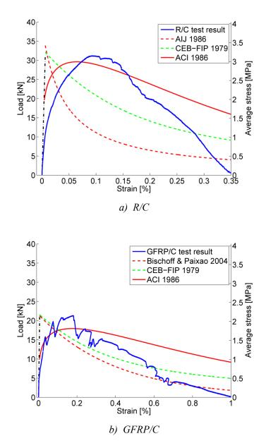
Figure 4-19 The tension stiffening effect of: a) R/C and b) GFRP/C in comparison to different tension stiffening model perditions.
