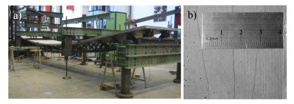
Figure 6-11 a) Deformed shape of specimen MP2 during ULS loading, and b) example of multiple flexural cracks on bottom of ECC slab at mid-span.
