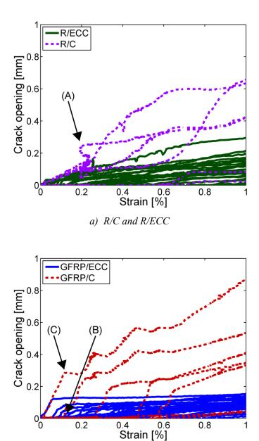
Figure 4-9 Development of crack opening vs. strain in a): R/C in comparison to R/ECC, (A) indicates where strain is halted due to opening of a crack at another location. b): GFRP/C in comparison to GFRP/ECC. (B) shows the formation of a new crack while (C) indicates where further crack opening is suspended due to (B).
