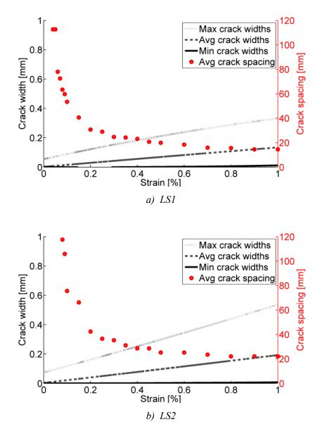
Figure 5-21 Average crack spacing in comparison to maximum, average and minimum crack widths compared with development of crack spacing as a function of tensile strain for a): LS1 and b): LS2.
