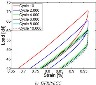
Figure 4-11 Cyclic loading hysteresis for a representative GFRP/ECC tension member loaded to 10.000 cycles. a) Overall cyclic response, b) close-up view of the upper end of the response shown in a).
