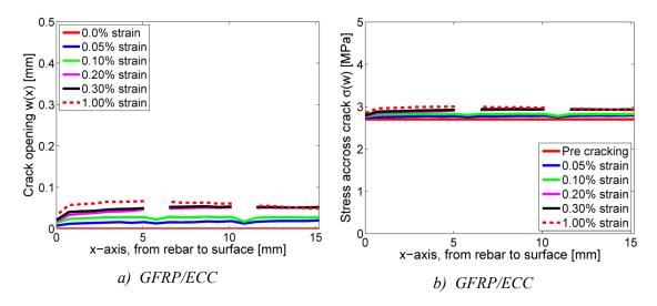
Figure 3-11 a): Crack opening profile for a transverse crack in GFRP/ECC at different strain levels and b): the corresponding stress transfer across the crack based on the cohesive law for ECC in tension,  $\sigma_{ECC}(w)$ , shown in Figure 3-2 and fracture mechanical parameters given in Table 3-1.
