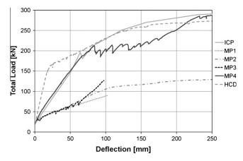
**Fig. 16.** Deflection at mid-span as a function of the total load of specimens MP1, MP2, MP4, ICP and the hollow core deck panel (HCD). Loading starts at 20 kN due to test configuration.
