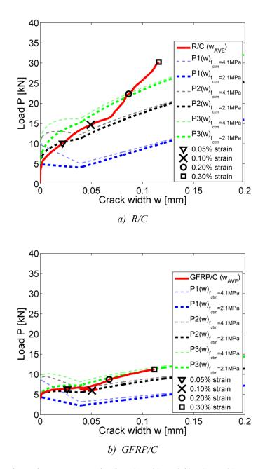
Figure 3-22 Load-crack opening results for a): R/C and b): GFRP/C in comparison to the three variations of the analytical solutions for the load-crack opening relationships given by equation 3.16 (P1, P2 and P3). Test results are shown up to a rebar strain of 0.3% with a: triangle, cross, circle and square markers indicating: 0.05%, 0.1%, 0.2% and 0.3% rebar strain respectively.
