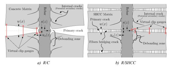
Figure 3-6 Schematic illustrations of deformations around reinforcement in a): R/C and b): R/SHCC (R/ECC).
