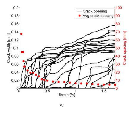
Figure 5-5 a) Stress – strain response of three dogbone-shaped tensile specimens in direct tension. b) Development of crack opening and crack spacing as a function of tensile strain obtained with DIC.
