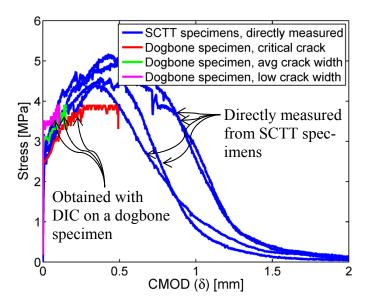
Figure 2-9 Examples of stress – crack mouth opening displacement ( $\sigma$  – CMOD) responses obtained from four SCTT specimens and comparison to the measurements obtained with DIC on a dogbone specimen. The critical crack in the dogbone specimen is the crack that ultimately localizes.
