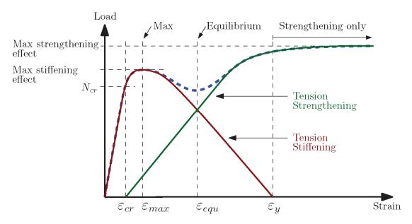
Figure 4-16 Conceptual model for the tension strengthening and stiffening process.
