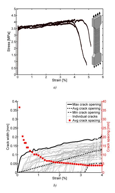
Figure 4-3 a) Stress-strain responses of three dogbone-shaped ECC tensile specimens in direct tension. b) Development of crack opening and crack spacing as a function of tensile strain obtained with DIC.
