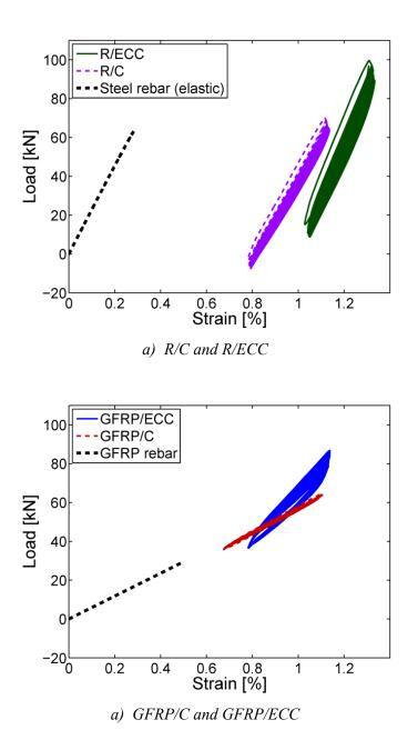
Figure 4-10 Cyclic loading hysteresis for: a) representative R/C and R/ECC and b) representative GFRP/C and GFRP/ECC tension members during 1000 cycles. The bare elastic response of the steel rebar and the bare response of the GFRP rebar up to 0.5% strain are shown for comparison.
