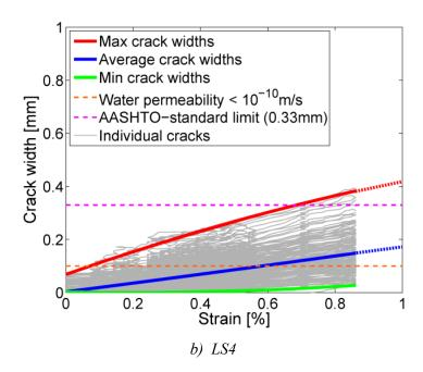
Figure 5-20 Development of crack opening as a function of strain during tensile loading of a): LS3 and b): LS4. The AASHTO crack width limit of 0.33 mm for highway bridges (AASHTO, 2002) is shown for comparison as well as the threshold for water permeability of 10<sup>-10</sup> m/s (Wang et al., 1997).
