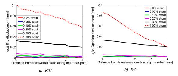
Figure 3-14 Debonding displacement profiles resulting from a transverse crack in R/C, a): sliding displacement, slip s(z), and b): opening displacement,  $u_x(z)$ , at different rebar strain levels.
