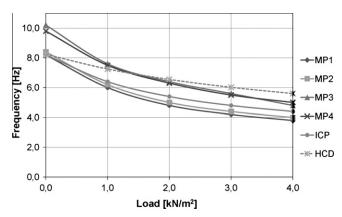
Fig. 14. The measured natural frequency as a function of applied service load.
