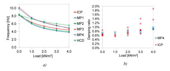
Figure 6-8 a) The measured natural frequency as a function of applied service load, and b) Measured damping ratios for specimens MP4 and ICP as a function of applied service load.
