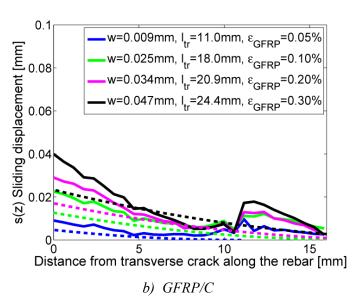
Figure 3-21 Comparison between theoretical slip values obtained from equation 3.13 (dashed lines) and the actual measured global slip s(z) values (continuous lines) for a):
