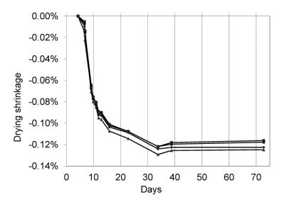
Figure 6-6 Drying shrinkage measurements of ECC.
