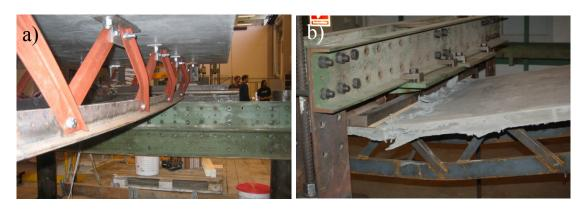
Figure 6-10 a) Buckling of compression diagonals in specimen MP1, and b) A combination of compression and flexural failure during ULS testing of specimen MP4.
