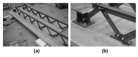
Fig. 11. (a) Steel truss assembly. (b) Bolted connection to ECC slab.
