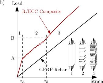
Figure 5-4 Schematic illustration of the tension stiffening process and crack formation in: a) GFRP reinforced concrete (GFRP/C) and b) GFRP reinforced ECC (GFRP/ECC). " $P_A$ " and  $\varepsilon_A$  are load and corresponding strain of first crack respectively, and " $P_B$ " and  $\varepsilon_B$  are load and strain after crack saturation occurs respectively.
