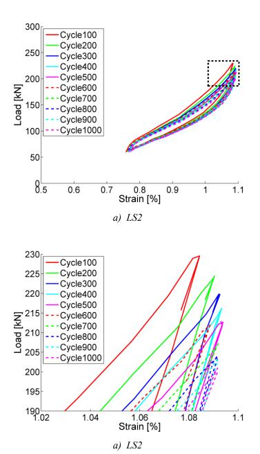
Figure 5-16 Load-strain hysteresis from cyclic testing of LS2. a): overall cyclic response and b): enlarged crest of the hysteresis.
