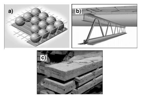
Fig. 2. Commercially available floor systems: (a) Bubble deck in Principe [7], (b) Hambro deck system in principle [11]. (c) Timber-concrete composite slab system [12].
