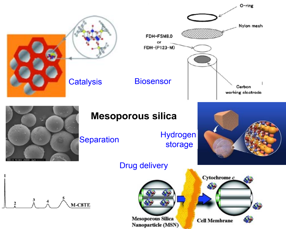
Fig. 2.4 Schematic illustration of some examples for promising applications of mesoporous silica. (Biosensor); FDH: formaldehyde dehydrogenase, FSM8.0: A folded-sheet mesoporous silica material having honeycomb structures with ordered cylindrical channels of 8.0-nm diameter, P123-M: An alumina membrane comprising surfactant (Pluronic P123)-templated silica nanochannels with a channel diameter of 8.0 nm within the columnar alumina pores [34]. (Separation); M-C8TE: MCM-41 modified with n-octyltrimethoxysilane and endcapped with hexamethyldisilazane [35]. Images are obtained from [36] (Catalysis); [34] (Biosensor); [33] (Hydrogen storage); [37] (Drug delivery); and [35] (Separation).
