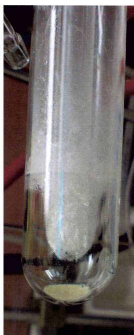
Figure 6. Sublimation of ‘crude’ FDMC from the oxidation reaction of HMF in methanol to afford colourless crystals of pure FDMC.
